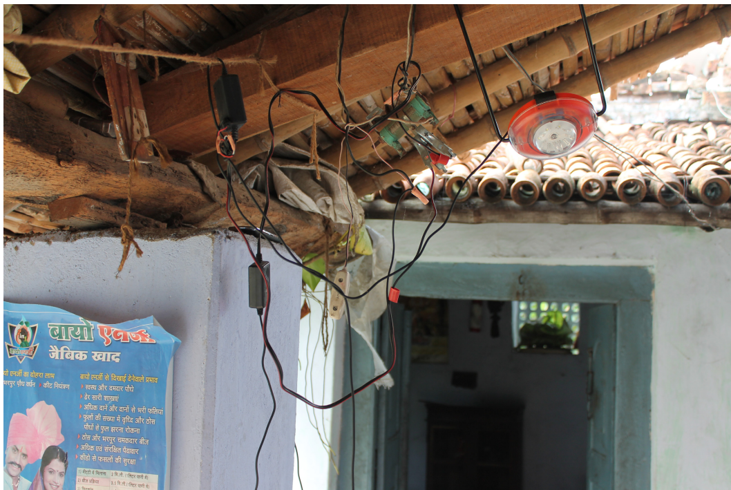
FIGURE 4 Mobile phone being charged after modifying a SK lamp meant to produce only light into a solar phone charger (Author, 2012).
