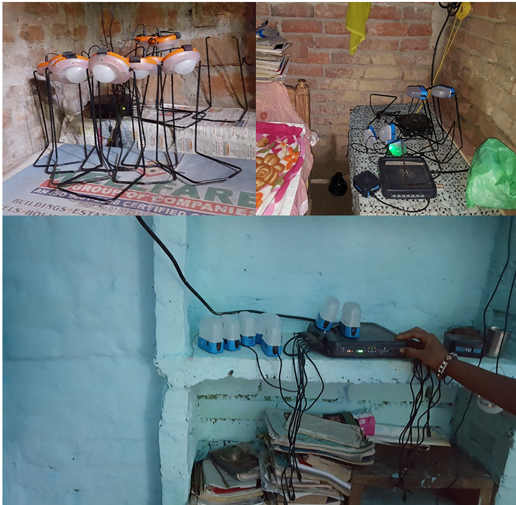
FIGURE 1 Old VL kit with SK lamps in VL kit in 2016 (top left). VL kit after SK lamps were replaced and the villagers demanded stands in 2017 (top right). VL kit in a new village in 2017 where people had not experienced SK lamps (bottom). In the bottom picture from right to left—cube, router and lamps (Author, 2016, 2017).
