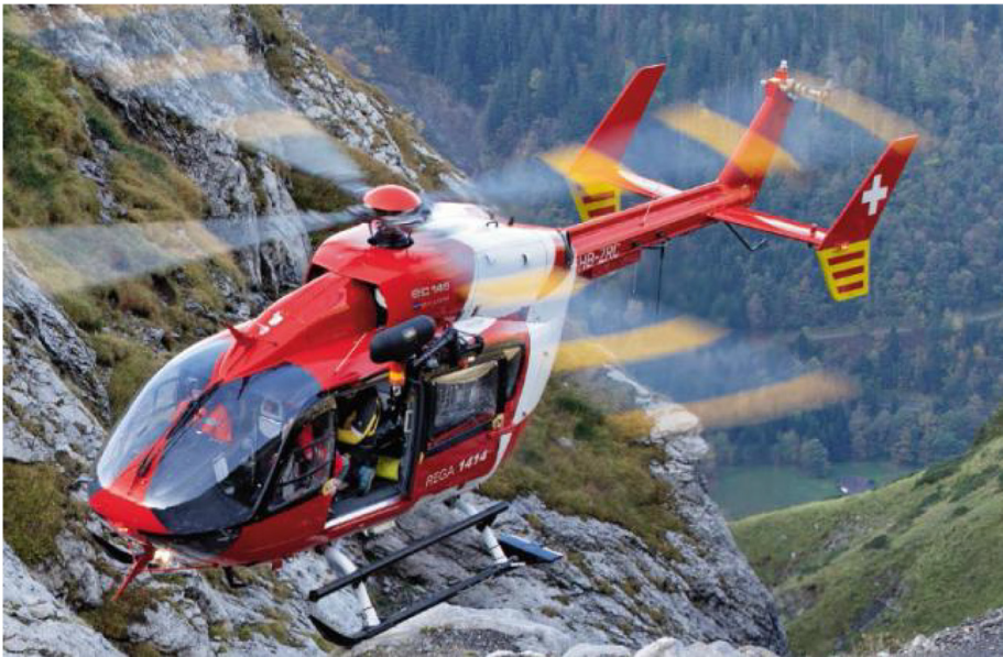
Figure 6. EC145 of the HEMS operator Rega. The GPS antenna is attached on the top of the fin in front of the strobe light (courtesy Rega).
