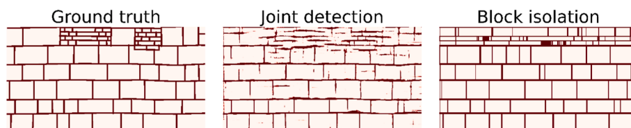
Fig. 13. Masonry joint segmentation before and after application of joint fitting algorithm.
