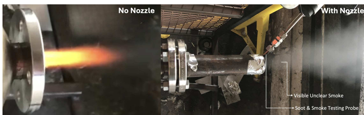
Figure 10. Initial Jet–A1 tests with visible smoke.
