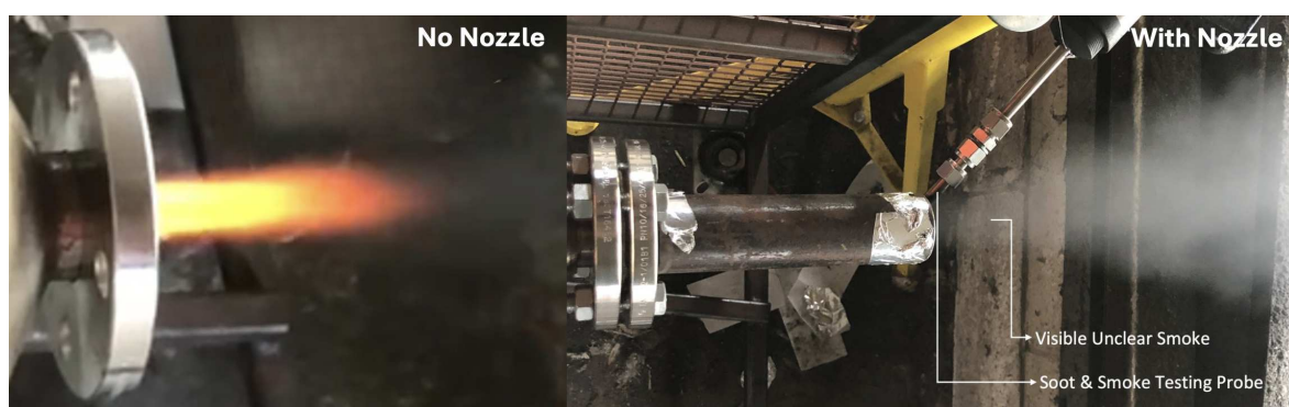
Figure 10. Initial Jet–A1 tests with visible smoke.
