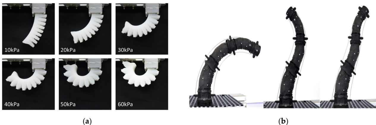
Figure 15. Building block-based soft robots: (a) The bellows block is actuated by high-pressure air [93]; (b) The soft robot includes the tendon-driven tube blocks [59].
