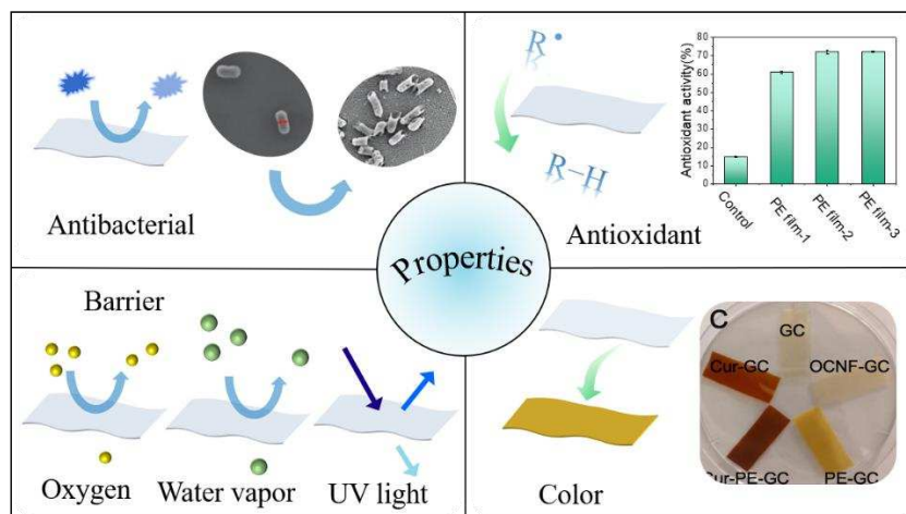
Fig. 6. Diagram illustrates the antibacterial [Reprinted with permission from (Gao et al., 2020). Copyright 2020 The Royal Society of Chemistry], antioxidant, barrier and color properties [Reprinted with permission from (Jian Liu et al., 2022). Copyright 2022 Elsevier] of Pickering emulsion-based composite films.
