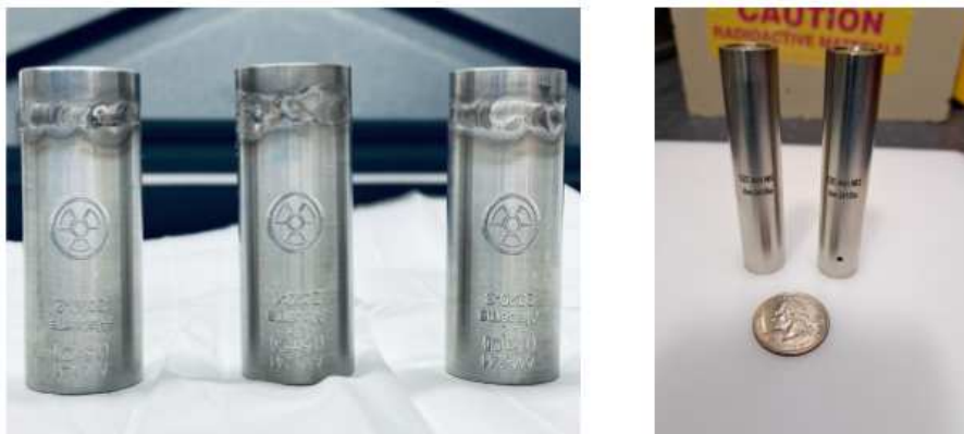
Figure 13. Left: three custom-made AmLi sources used in LZ. The gold-americium-lithium matrix is encapsulated in nested tungsten and stainless steel capsules, which are designed to integrate with the CSD system and provide gamma-radiation suppression. The welds on the outer stainless-steel capsules are visible in the picture. Right: two customized AmBe sources from Eckert & Ziegler designed for LZ. The stainless steel threaded capsules were designed to integrate in the CSD system and shield against low energy gammas from ^{241}\text{Am} decay.
