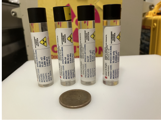
Figure 15. Picture of ^{57}\text{Co} , ^{54}\text{Mn} , ^{22}\text{Na} , and ^{228}\text{Th} \gamma -ray sources that are deployed in LZ for high energy ER calibrations.
