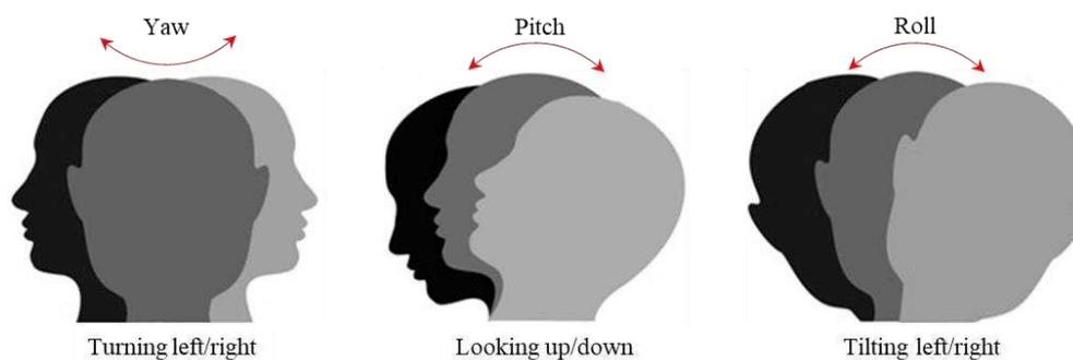
Figure 4. Scheme of head movement around yaw, pitch, and roll axes
