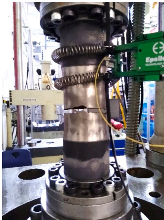
Fig. 6. Image showing a failed tensile test specimen. Note that the extensometer was repositioned for the photograph.
