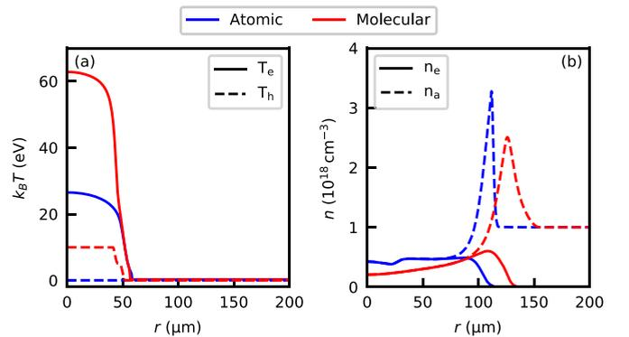
FIG. 6. Effects of molecular hydrogen on the example simulation of HOFI channel formation from a Gaussian HOFI pulse shown in Sec. III. (a) The initial temperature profiles resulting from the atomic and the rapid molecular ionization models. (b) The density profiles after 2 ns of expansion in the HYQUP simulation. For the molecular case, the background gas is changed to initially be molecular.
