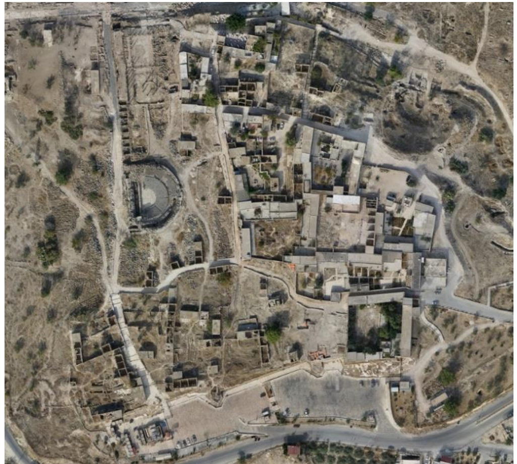
Figure 8. Drone-mounted generated orthomosaic plan. Accuracy 25–30 mm.
