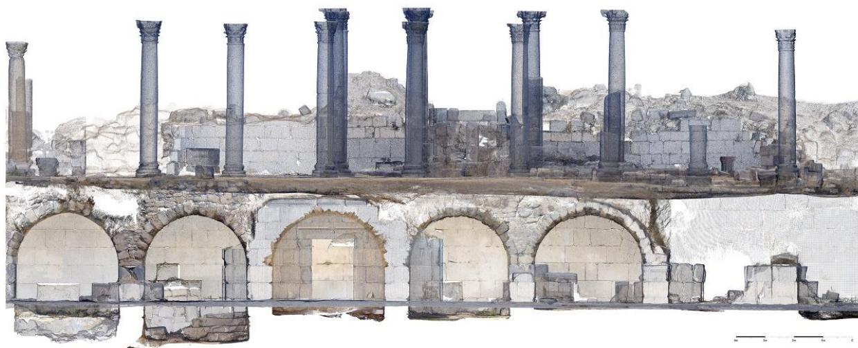
Figure 6. The central section of the north–south elevation image of the Byzantine monuments on the earlier Roman terrace showing the Byzantine octagonal centralised church above the Roman Cardo street and vaulted shops of ancient Gadara. Image generated from the cleaned 3D point cloud.
