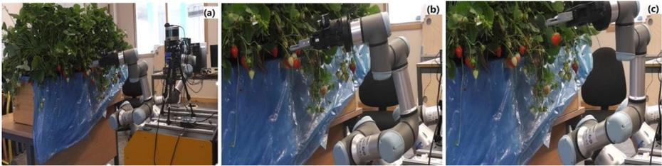
**Fig. 15** Test of the action system in a Lab setting: (a) the arm reaches the target position; (b) the gripper has cut the stem of the target strawberry; (c) the gripper remains closed until it goes to the specified position
