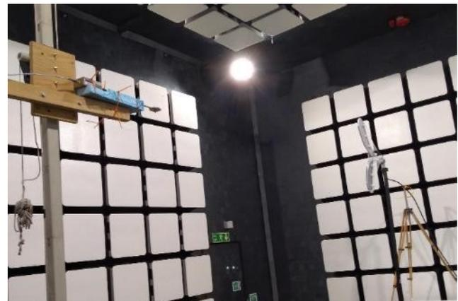
Fig. 21. Hyperband antenna under test (right) in anechoic chamber, showing D-dot probe (left)
