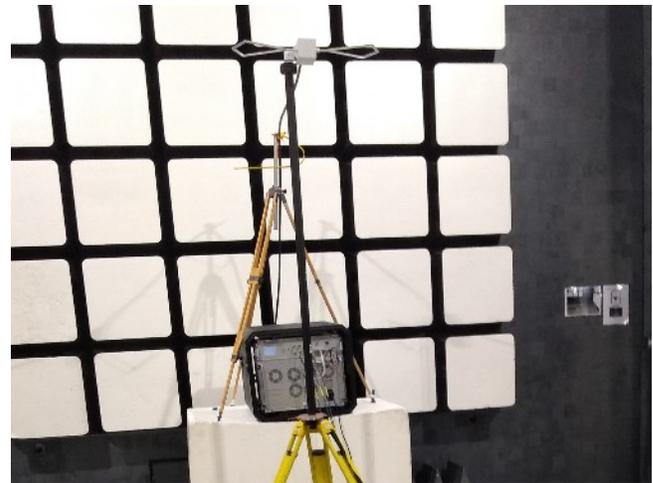
Fig. 29. 150 MHz Antenna under test in anechoic chamber with pulse generator below
