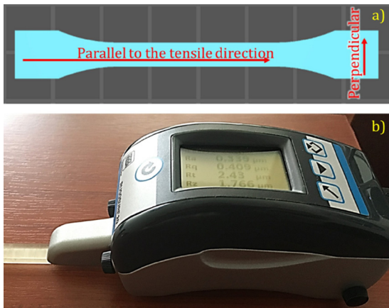
Figure 6. a) Surface roughness measuring directions, b) measurement process.
