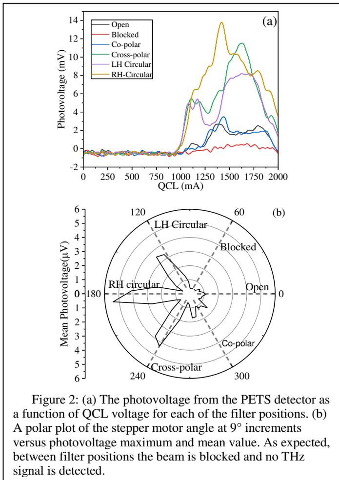
Figure 2: (a) The photovoltage from the PETS detector as a function of QCL voltage for each of the filter positions. (b) A polar plot of the stepper motor angle at  $9^\circ$  increments versus photovoltage maximum and mean value. As expected, between filter positions the beam is blocked and no THz signal is detected.
