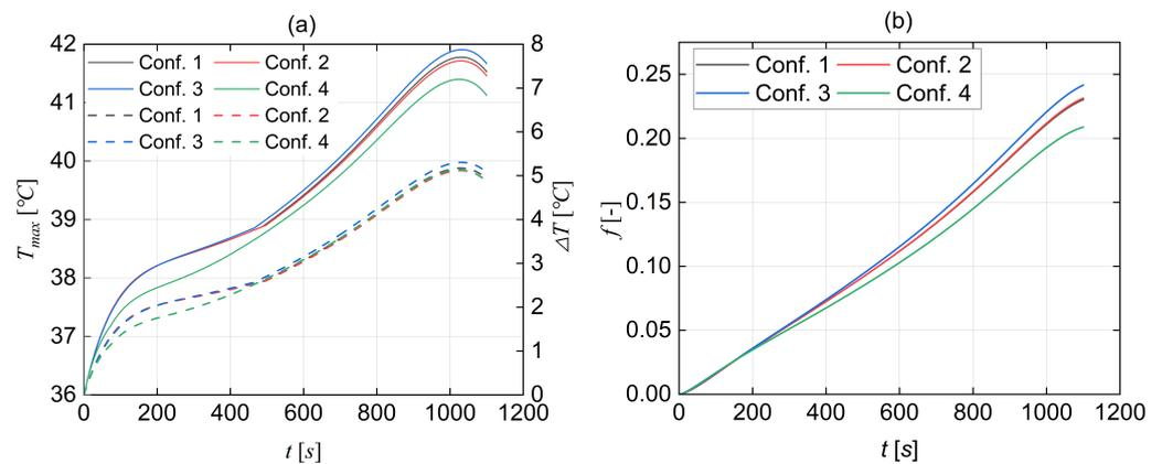
**Figure 9.** Results of four different configurations (Conf.#) at a temperature of 36 °C and the 3 C rate of the cell using CPCM-3 showing (a) maximum temperature (solid lines) and temperature difference (dashed lines), and (b) liquid fraction, over time.
