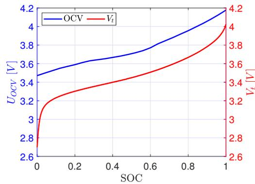
**Figure 1.** Experimental measurements of OCV, and the terminal voltage as a function of SOC at the end of 3 C discharge (at 25 °C)—adapted with permission from [28].
