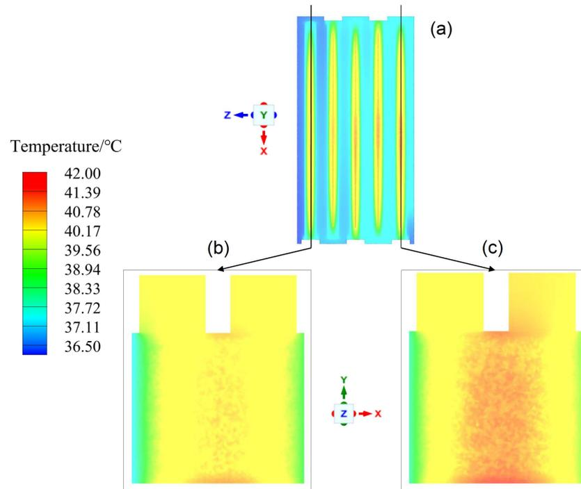
**Figure 8.** Temperature distribution of configuration (1) at 3 C discharge rate and using CPCM-3 (a) from the top view of the LIB pack, (b) of the LIB near the coolant inlet, and (c) of the LIB near the coolant outlet.
