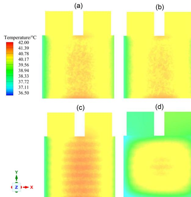
**Figure 11.** Temperature distribution along the longitudinal interface of the LIB pack closet to the coolant outlet at 3 C discharge rate and using CPCM-3 for (a) configuration (1), (b) configuration (2), (c) configuration (3), and (d) configuration (4).
