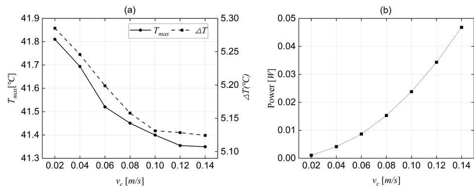
**Figure 12.** Cooling performance and energy consumption of BTMS at different coolant flow rates—at 3 C discharge rate and using CPCM-3—indicating (a) BTMS cooling performance (maximum temperature and maximum temperature difference), and (b) BTMS energy consumption.
