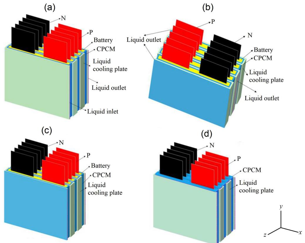
Figure 4. Four different BTMS configurations analysed in this study, (a) configuration (1), (b) configuration (2), (c) configuration (3), and (d) configuration (4).
