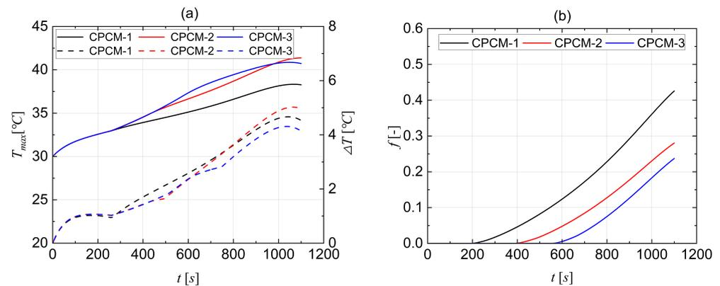
**Figure 6.** Results at a temperature of 26.85 °C and the 3 C rate of the cell showing (a) maximum temperature (solid lines) and temperature difference (dashed lines), and (b) liquid fraction, over time.
