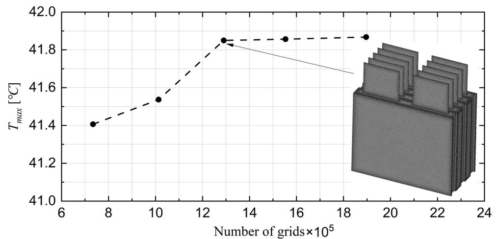
**Figure 5.** Mesh independence of the 3-D model with respect to the number of grids, and an example of mesh topology.
