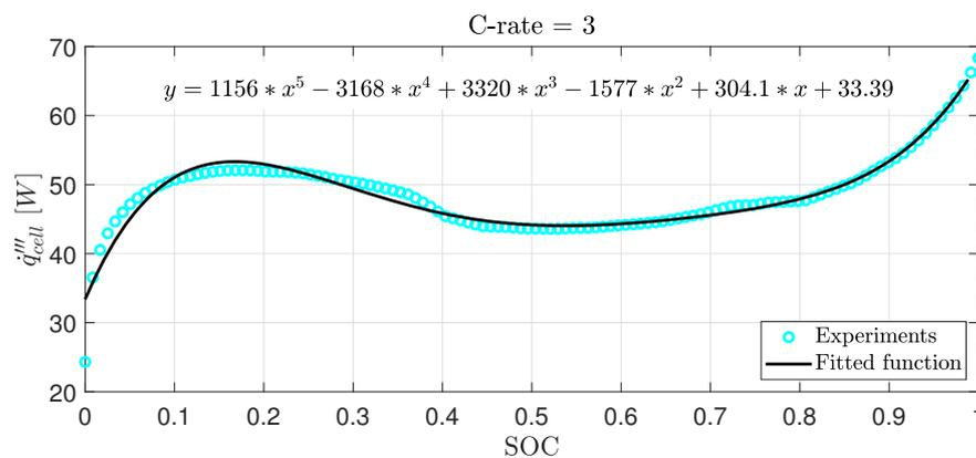
**Figure 2.** Heat generation curve inside a 53 Ah LIB cell (with a natural convection state,  $h_\infty = 6 \text{ W/m}^2\cdot\text{K}$ ) and the corresponding fitted functions at discharge rate of 3C — adapted with permission from [30].
