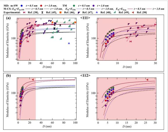
**Figure 3.** The modulus of elasticity, E, for aSiO<sub>2</sub>-Si NWs in (a)  $\langle 111 \rangle$  and (b)  $\langle 112 \rangle$  crystal orientations. MD simulations are used to predict the  $E_{\rm Si}$  along with experimental values while combined with M-CS model of this work. Experimental data [38, 45–50] is plotted by extracting the modulus of elasticity (E) from each respective study and utilizing it in the analysis of E as a function of D.
