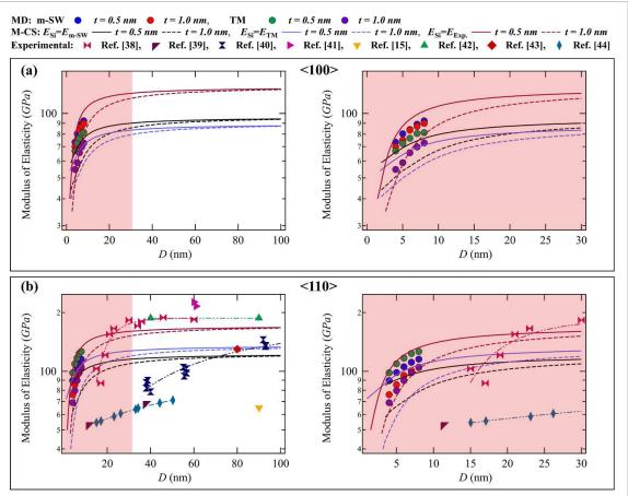
**Figure 2.** The modulus of elasticity, E, for aSiO<sub>2</sub>-Si NWs in (a)  $\langle 100 \rangle$  and (b)  $\langle 110 \rangle$  crystal orientations. MD simulations are used to predict the  $E_{Si}$  along with experimental values while combined with M-CS model of this work. Experimental data [14, 38–44] is plotted by extracting the modulus of elasticity (E) from each respective study and utilizing it in the analysis of E as a function of D.
