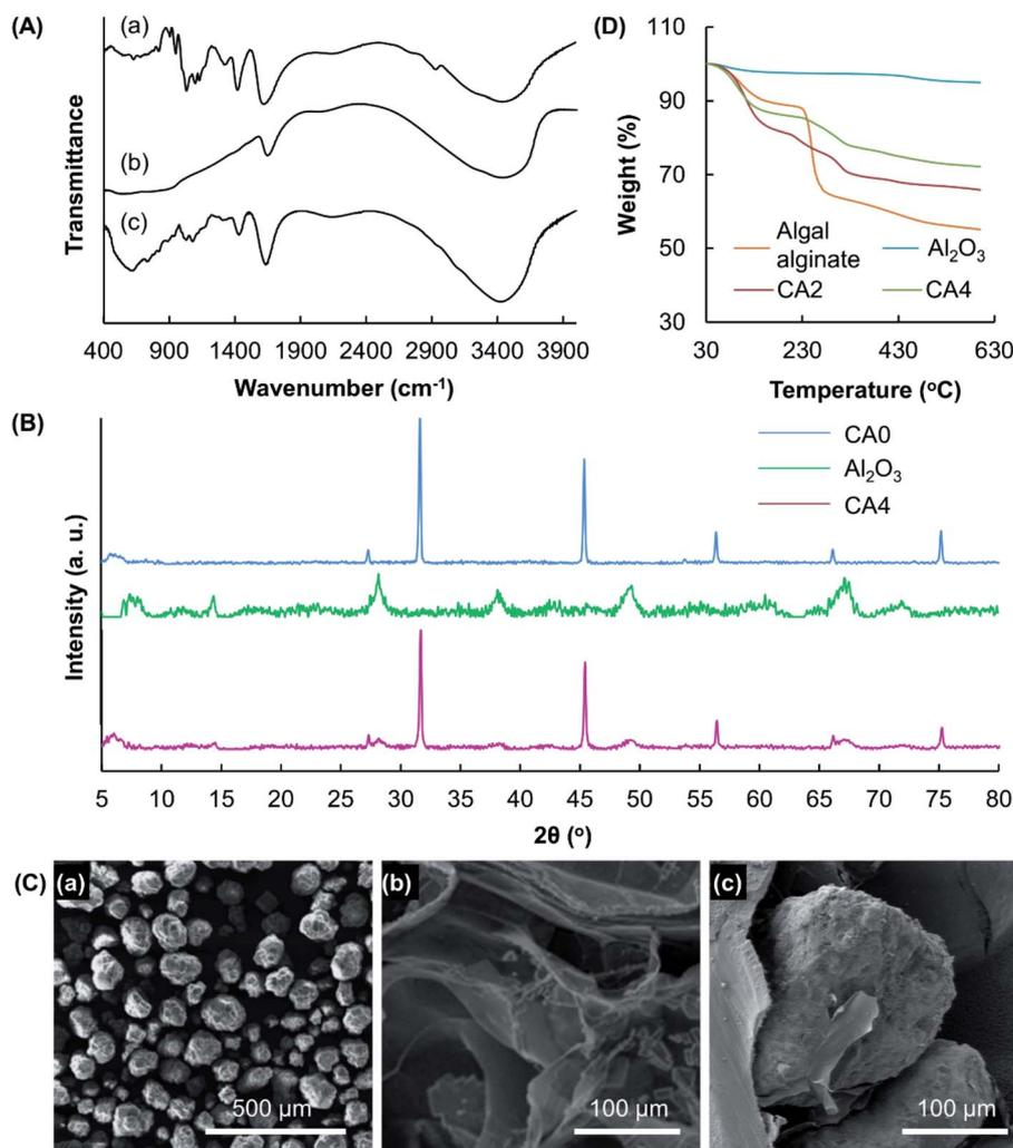
Fig. 3 (A) FT-IR spectra of (a) algal alginate, (b)  $\text{Al}_2\text{O}_3$ , and (c) CA4. (B) XRD patterns of  $\text{Al}_2\text{O}_3$ , CA0 and CA4. (C) SEM micrographs of (a)  $\text{Al}_2\text{O}_3$  and (b) CA0, and (c) a magnified view showing the presence of  $\text{Al}_2\text{O}_3$  incorporated into the gel matrix of CA4. (D) TGA curves of algal alginate,  $\text{Al}_2\text{O}_3$ , CA2 and CA4.
