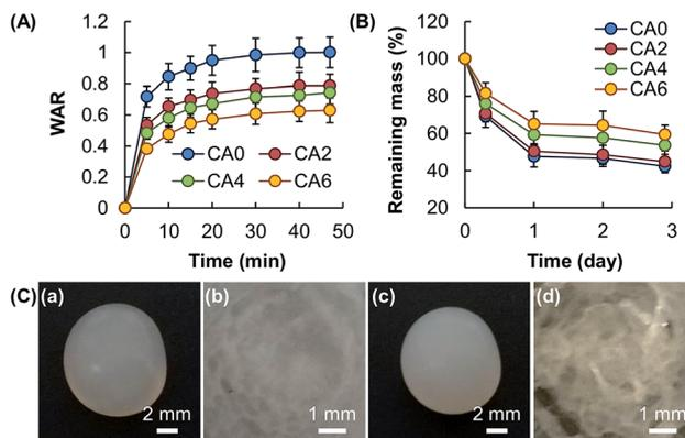
Fig. 5 (A) The swelling capacity and (B) erosion susceptibility of hydrogel beads consisting of CA0, CA2, CA4, and CA6. Data are presented as the means  $\pm$  SD of triplicate experiments. (C) Photos of (a, c) a hydrogel bead consisting of CA0 and (b, d) a magnified view of the cross-section of the bead after lyophilization. The photos are taken (a, b) before and (c, d) after immersion of the bead in simulated body fluid for 1 day.
