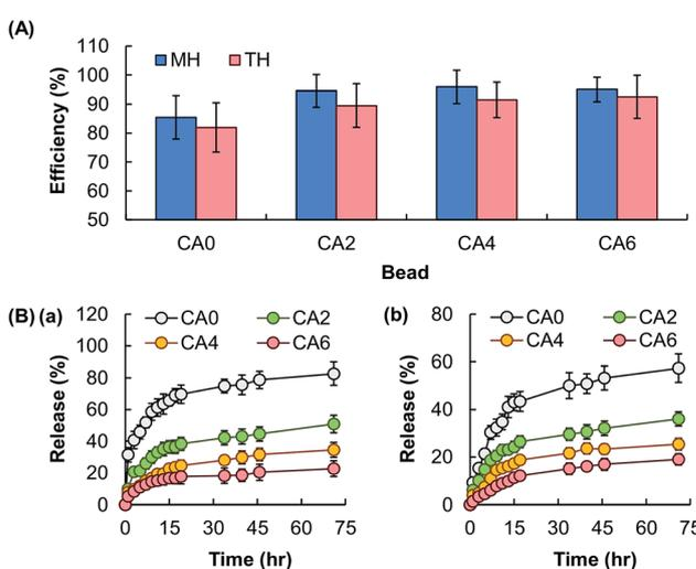
Fig. 6 (A) The EE of hydrogel beads consisting of CA0, CA2, CA4, and CA6. Data are presented as the means  $\pm$  SD of triplicate experiments. (B) The profiles of release of (a) TH and (b) MH from hydrogel beads consisting of CA0, CA2, CA4, and CA6. Data are presented as the means  $\pm$  SD of triplicate experiments.
