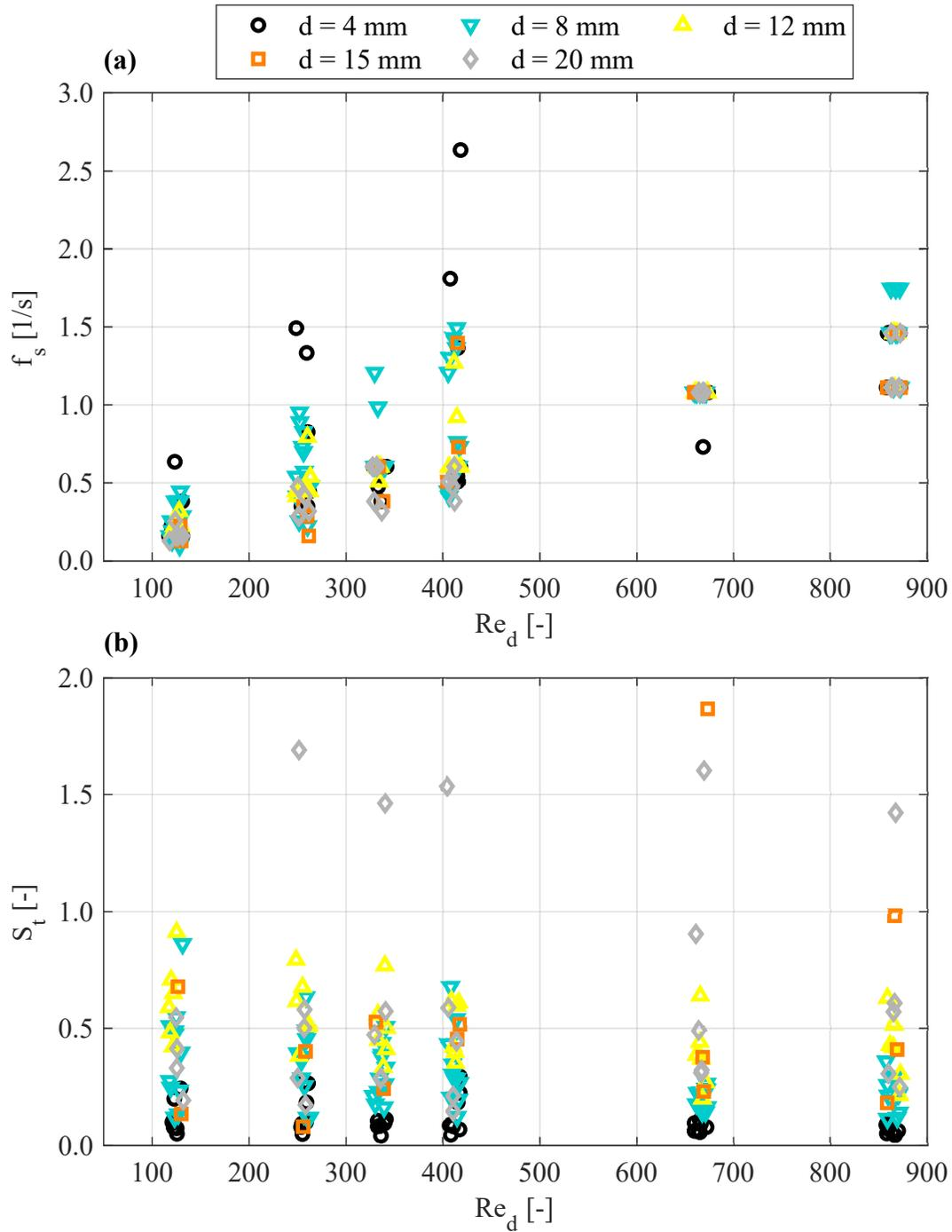
**Fig. 6.** a) Variation of shedding frequency,  $f_s$ , from the velocity spectra. b) Variation of Strouhal numbers, from shedding frequencies, using the reference cylinder diameter and local velocities as length and velocity scales, respectively.
