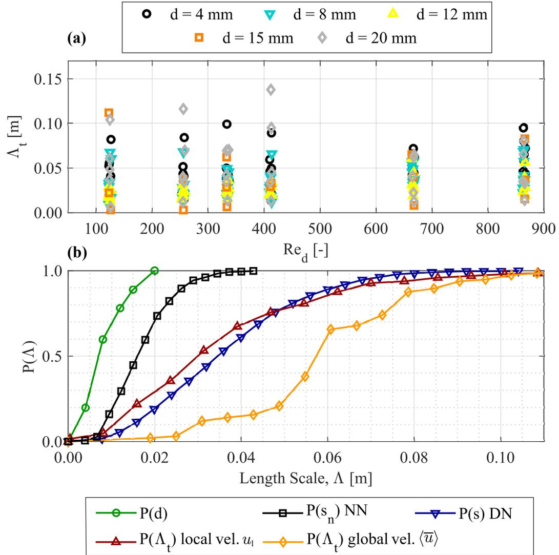
**Fig. 8.** a) Variation of point-based estimates of length scales,  $\Lambda_t$ , with respect to stem Reynolds number,  $Re_d$ , and b) density and cumulative Distribution functions for  $\Lambda_t$ , for local and global estimates of velocity.
