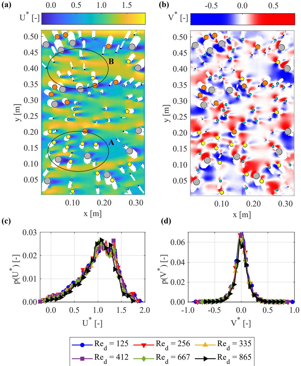
**Fig. 2.** Non-dimensional **a)** time-averaged streamwise velocity,  $U^*(x, y)$  and **b)** time-averaged transverse velocity,  $V^*(x, y)$  for  $Re_d = 335$ . Probability distribution of the time-averaged maps of non-dimensionalised **c)** streamwise and **d)** transverse velocities, for all  $Re_d$
