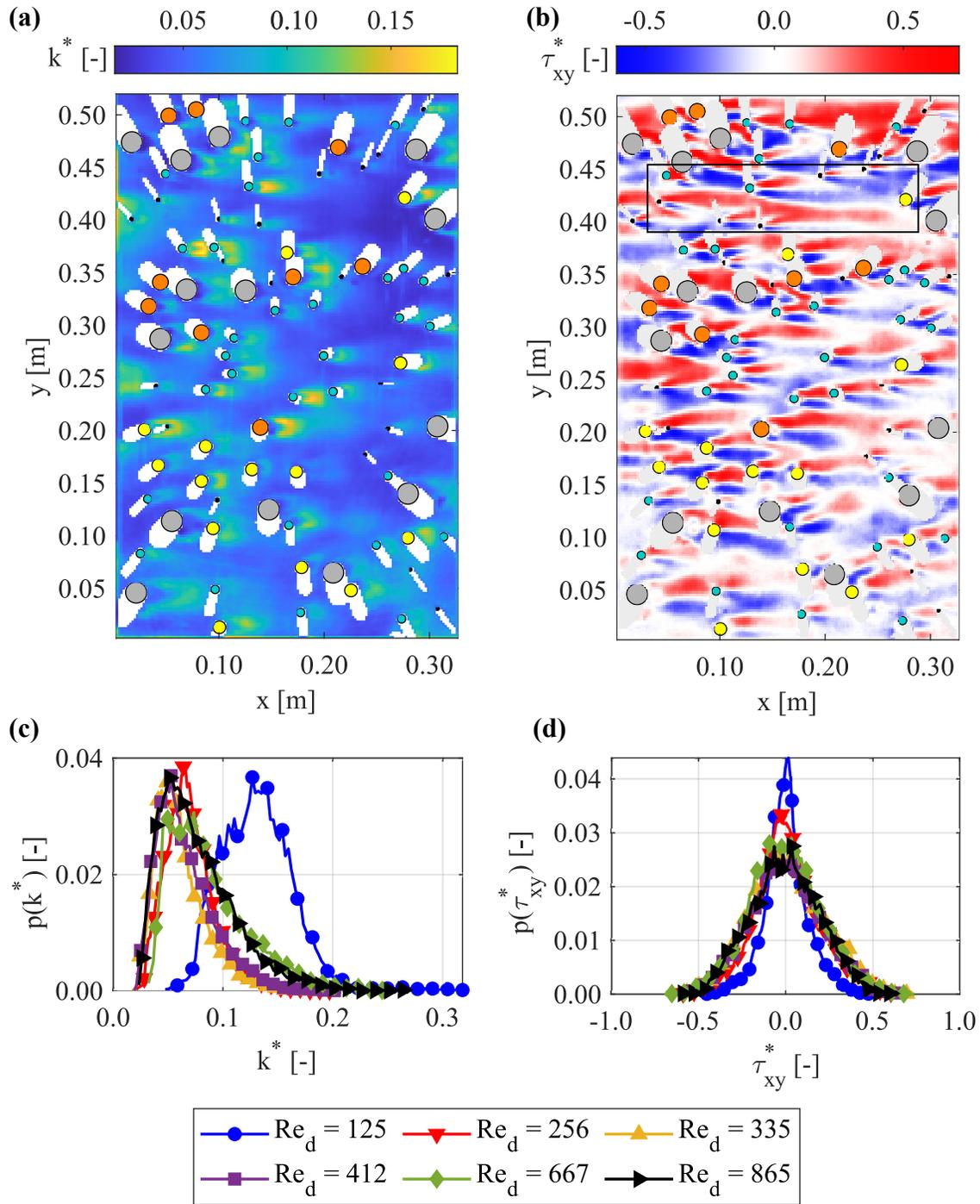
**Fig. 3.** Non-dimensional **a)** Turbulent Kinetic Energy,  $k^*(x, y)$  and **b)** shear Reynolds stresses,  $\tau_{xy}^*(x, y)$  for  $Re_d = 335$ . Probability distribution of the time-averaged maps of non-dimensionalised **c)** Turbulent Kinetic Energy and **d)** Shear Reynolds stresses, for all  $Re_d$
