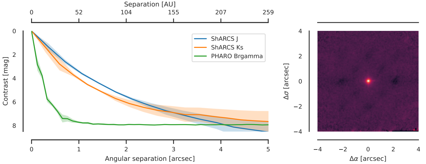
Fig. 1. Contrast with its 1\text{-}\sigma uncertainties as a function of separation and angular separation in Brgamma, J and Ks (left) and a high-resolution PHARO image (right).
