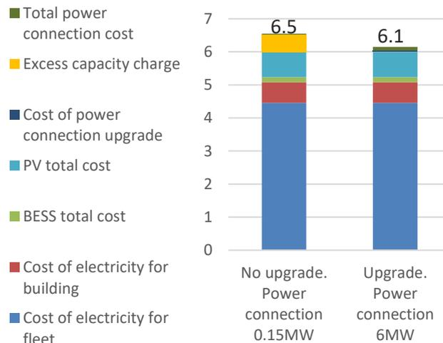
Fig. 8 (b) Total cost over system lifetime for scenario 2 (PV+BESS+eRCVs) when the fleet is charged at 16:00h
