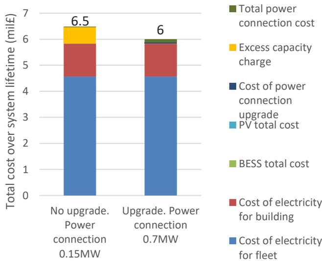
Fig. 14 (a) Total cost over system lifetime for scenario 1 (Grid+eRCVs) when the fleet is charged at 11:00h & 23:00h.
