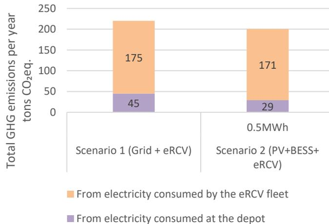
Fig. 12. Total GHG emissions per year for scenario 1 (Grid+eRCVs) and for scenario 2 (PV+BESS+eRCVs) when the fleet is charged at 21:00h.
