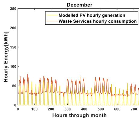
Fig. 4. Hourly electricity consumption and modelled PV solar energy generation during December.
