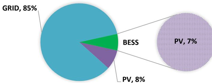
Fig. 10. Percentage of total demand covered by the grid and by the PV solar energy (instantaneous and stored energy at the BESS) when the fleet is charged at 21:00h.
