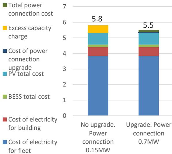
Fig. 14 (b) Total cost over system lifetime for scenario 2 (PV+BESS+eRCVs) when the fleet is charged at 11:00h & 23:00h.
