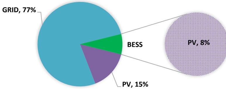
Fig. 13. Percentage of total demand covered by the grid and by the PV solar energy (instantaneous and stored energy at the BESS) when the fleet is charged at 11:00h & 23:00h.
