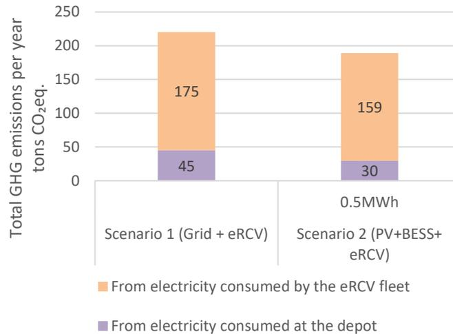
Fig. 15. Total GHG emissions per year for scenario 1 (Grid+eRCVs) and for scenario 2 (PV+BESS+eRCVs) when the fleet is charged at 11:00h & 23:00h.
