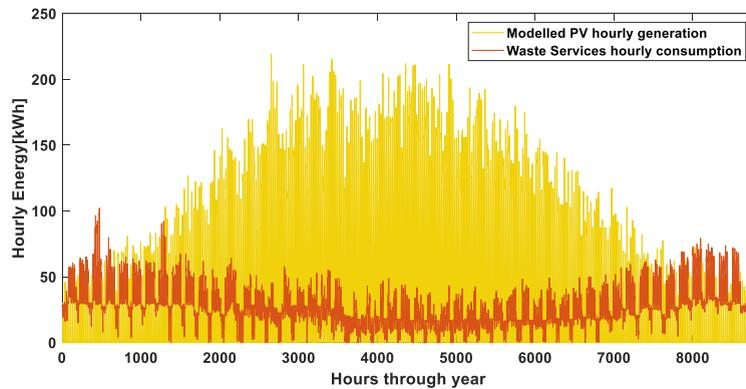
Fig. 3. Hourly electricity consumption and modelled PV solar energy generation for the depot under study.
