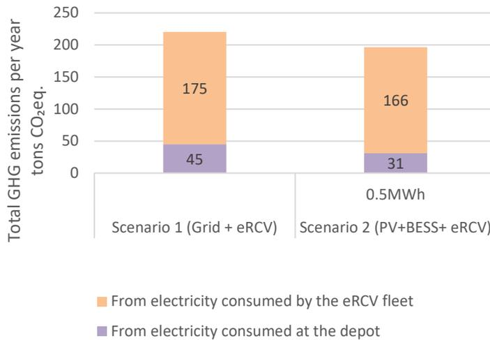
Fig. 9. Total GHG emissions per year for scenario 1 (Grid+eRCVs) and for scenario 2 (PV+BESS+eRCVs) when the fleet is charged at 16:00h.
