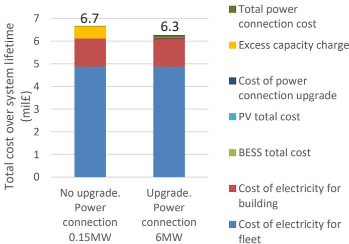
Fig. 8 (a) Total cost over system lifetime for scenario 1 (Grid+eRCVs) when the fleet is charged at 16:00h.
