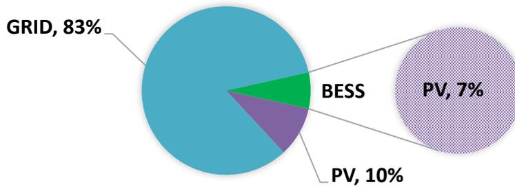
Fig. 7. Percentage of total demand covered by the grid and by the PV solar energy (instantaneous and stored energy at the BESS) when the fleet is charged at 16:00h.
