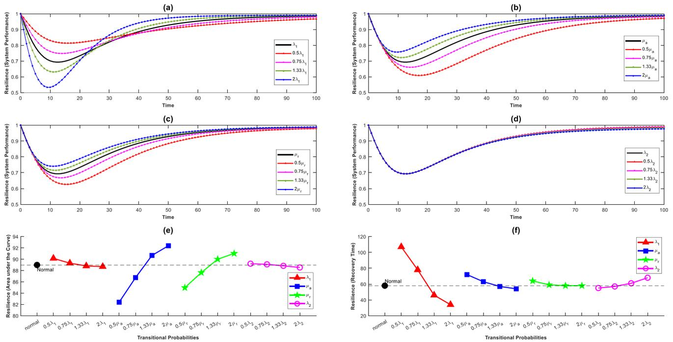
Fig. 12. Sensitivity analysis for transitional probabilities of  $\lambda_1$ ,  $\mu_a$ ,  $\mu_r$ , and  $\lambda_2$  at the late design stage.
