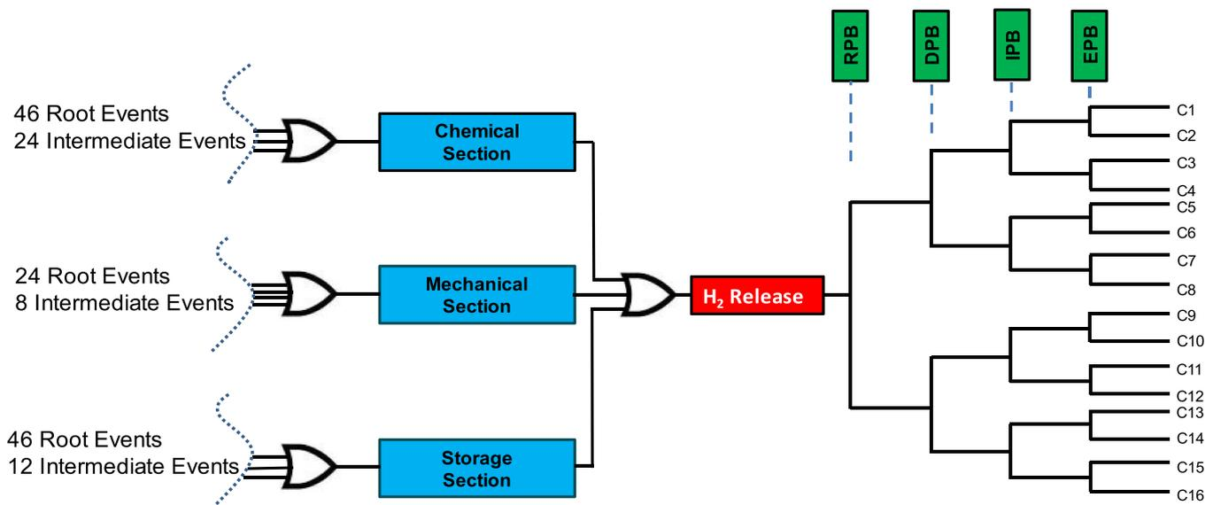
Fig. 10. The bow-tie diagram of the green hydrogen plant undergoing H<sub>2</sub> release scenarios.
