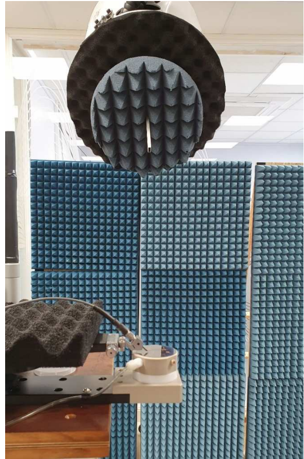
Fig. 8. Antenna undergoing radiated test on special mini prober station (phi sweep is vertically downwards as viewed here) [9].
