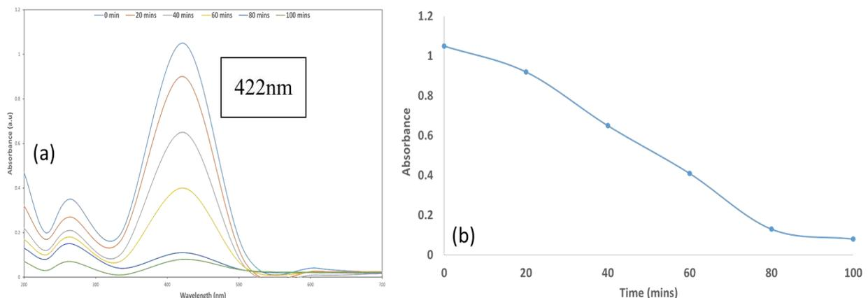
Figure 5: (a) UV-Vis spectra of methyl red degradation by using NaBH<sub>4</sub> and NiO NPs synthesised from Fragaria × ananassa (strawberry) and (b) Absorbance monitoring the decrease in methyl red intensity
