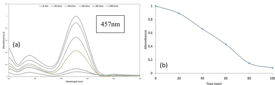
**Figure 7: (a) UV-Vis spectra of methyl red degradation by using NaBH<sub>4</sub> and NiO NPs synthesised from Citrus x paradisi (grapefruit) and (b) Absorbance monitoring the decrease in methyl red intensity**
