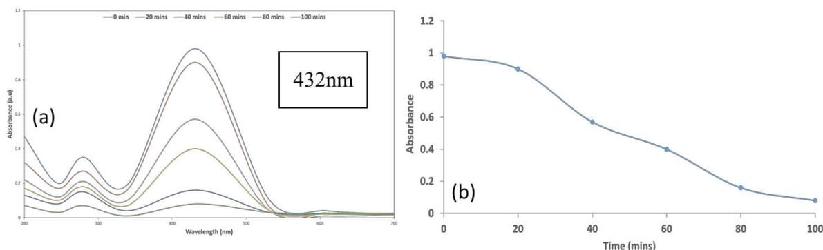
**Figure 6: (a) UV-Vis spectra of methyl red degradation by using NaBH<sub>4</sub> and NiO NPs synthesised from Vitis vinifera (grape) and (b) Absorbance monitoring the decrease in methyl red intensity**
