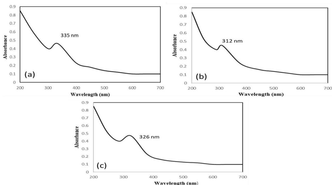
Figure 1: UV-Vis spectra of NiO NPs green synthesised by (a) *Fragaria  $\times$  ananassa* (strawberries) extract, (b) *Vitis vinifera* (grapes) extract, and (c) *Citrus  $\times$  paradisi* (grapefruit) extract
