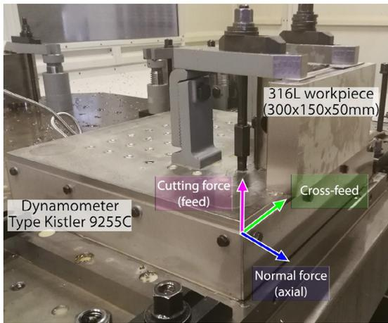
Fig. 2. Experiment setup for flood coolant and scCO<sub>2</sub> DoE Stage 2 on the Starrag HEC1800.
