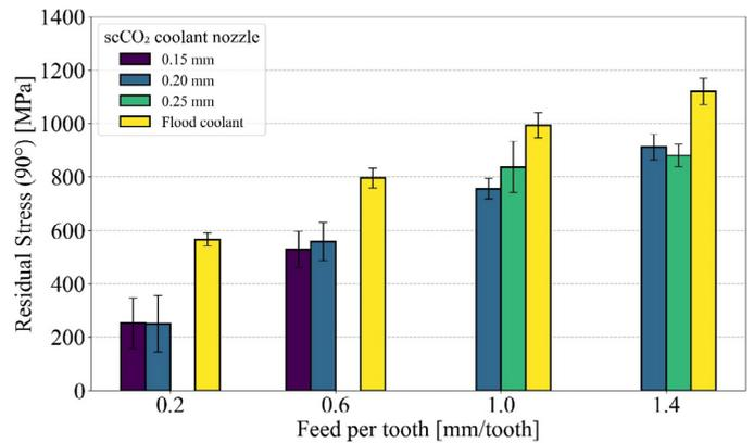
Fig. 9. Residual stress in longitudinal direction ( $\phi = 90^\circ$ ), with changes in feed per tooth and nozzle diameter.
