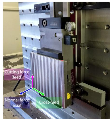
Fig. 1. Experiment setup for flood coolant and scCO<sub>2</sub> DoE Stage 1 on the Starrag HEC1800.
