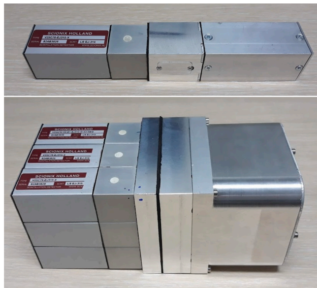
Fig. 7. Photos of one sTED module (top) and nine sTED modules grouped into a cluster (bottom).
