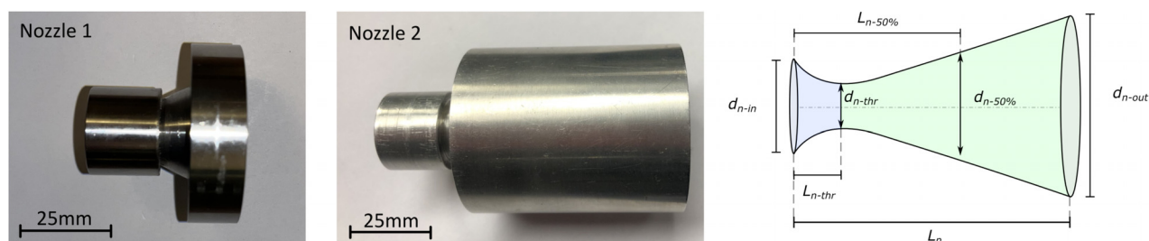
FIG. 3. Picture of nozzle 1 (left) and nozzle 2 (middle) used in experiments and a schematic of an arbitrary nozzle (right) profile with the main characterizing dimensions as shown in Table I. The blue-colored section refers to the converging section, and the green-colored section refers to the diverging section. Dimensions for nozzles used in this study can be seen in Table I.
