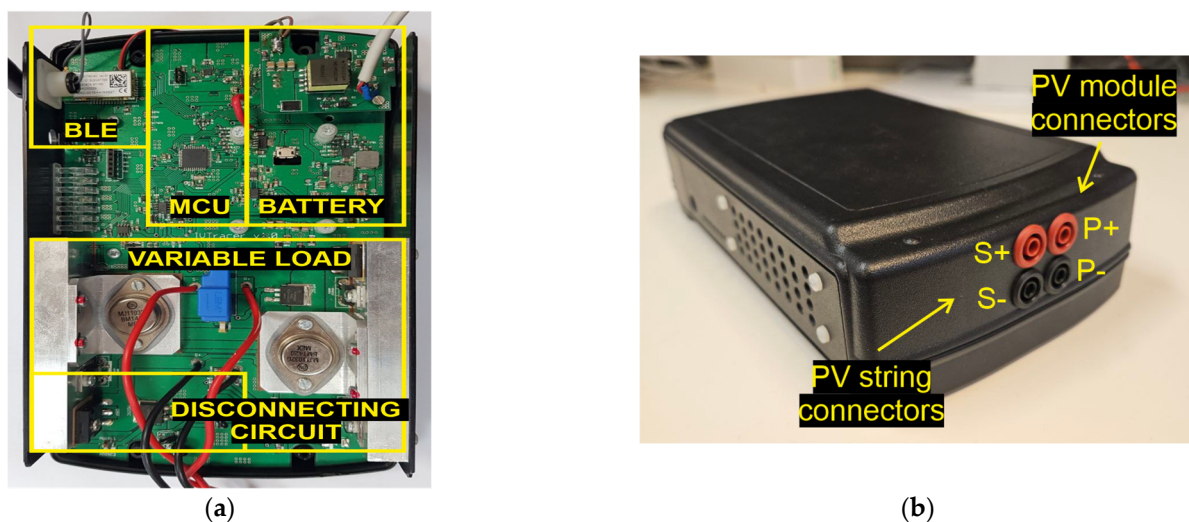
Figure 7. Physical layout of the developed I-V curve tracer. (a) The implemented prototype; (b) IP67-rated enclosure and connectors to PV module and PV string.
