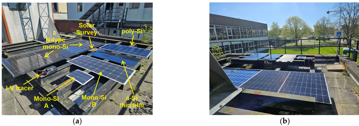
Figure 6. Experimental setup. (a) Tested PV panels; (b) outdoor experimental setup layout.
