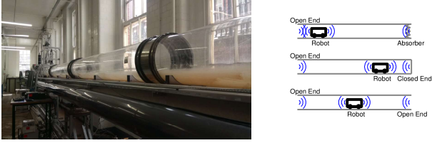
Fig. 1. A photograph of the pipe used to record experimental data, and an illustration of the robot within a pipe emitting a sound which echoes from the ends of the pipe. Three different scenarios are shown, which have been created experimentally. In all cases one end is open, and in each case the other end is open, closed, or filled with absorber, respectively.
