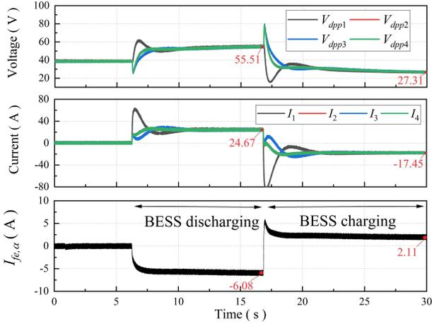
Fig. 13. Performance of the front-end and the DPP converters under high SoC condition
