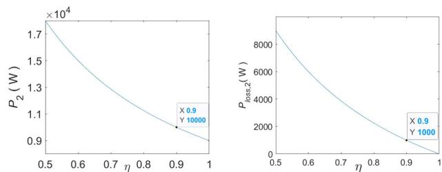
Fig. 16. The total power requirement and power loss of all converters with conventional configuration.
