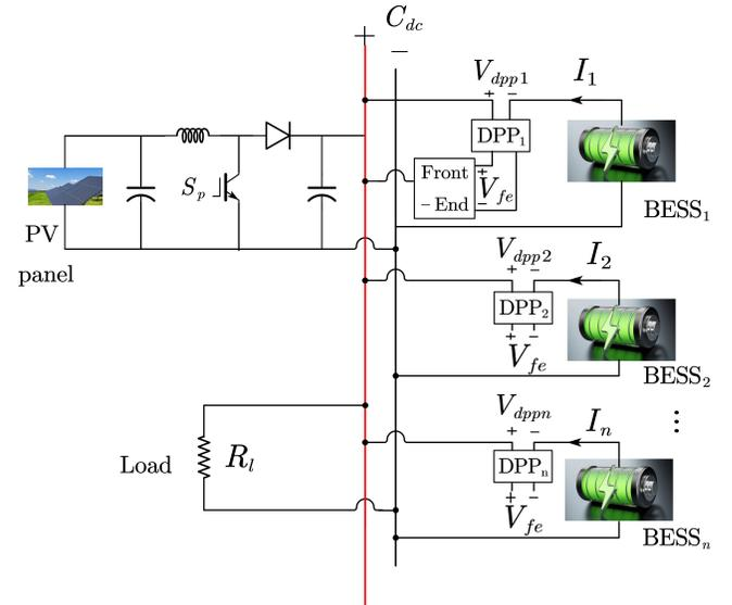
Fig. 3. The configuration of the DC microgrid in the proposed DPP-based control framework
