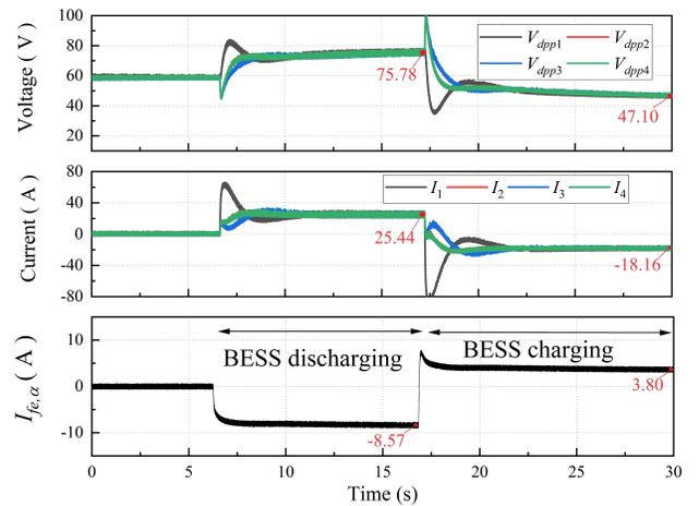
Fig. 12. Performance of the front-end and the DPP converters under low SoC condition
