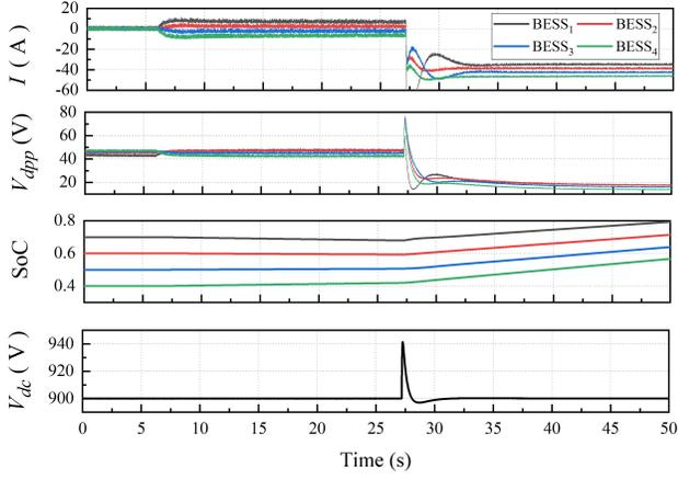
Fig. 9. BESSs SoC balance test when  $k=0.2$
