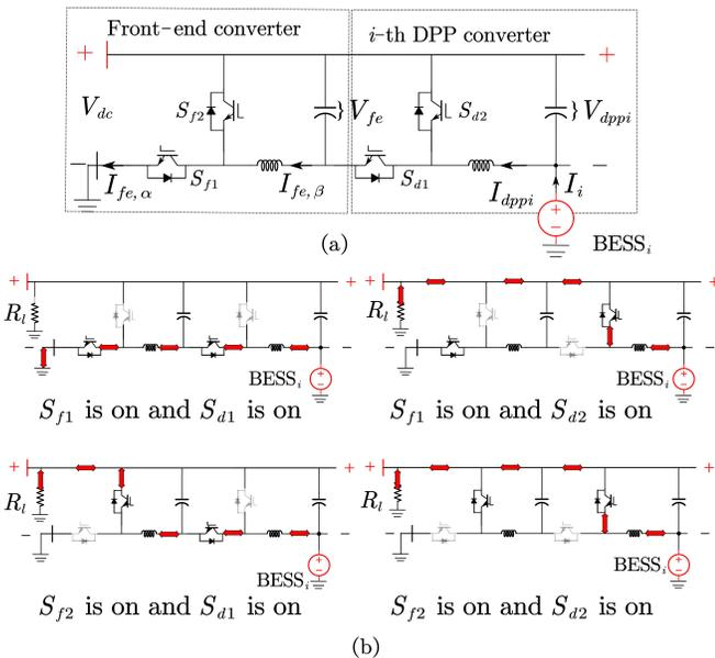
Fig. 4. Inverted bidirectional buck converters (a) topology (b) power flow analysis
