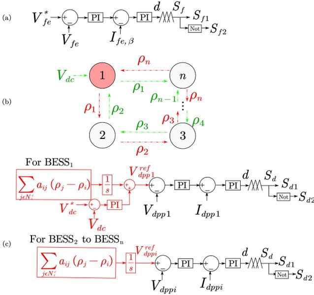
Fig. 5. The proposed control strategy (a) the front-end converter control algorithm (b) communication links (c)  $i$ -th DPP converter control algorithm
