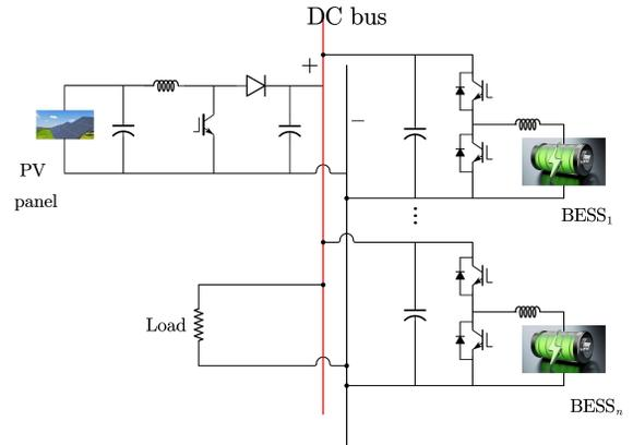
Fig. 1. Conventional BESS-DC bus configuration
