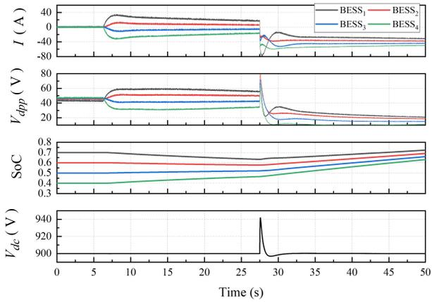
Fig. 10. BESSs SoC balance test when  $k=2$
