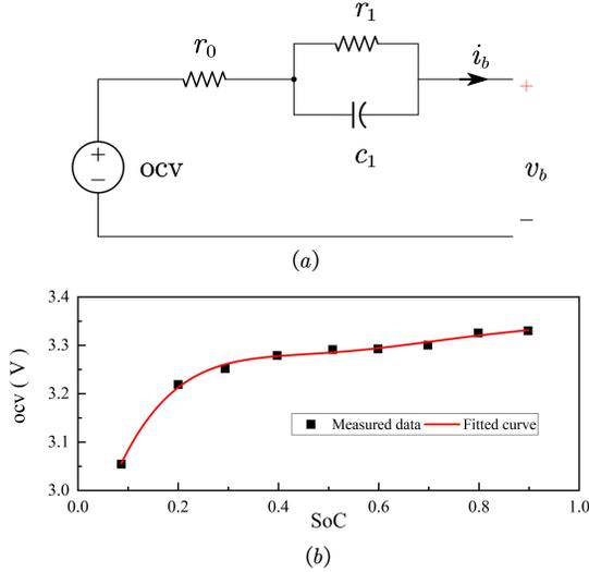
Fig. 2. Battery model (a) Equivalent circuit model (b) ocv versus SoC of  $\text{LiFeO}_4$  battery
