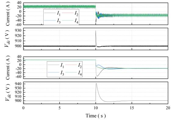
Fig. 14. The test results with the conventional configuration (first two figures) and the proposed control framework (last two figures)
