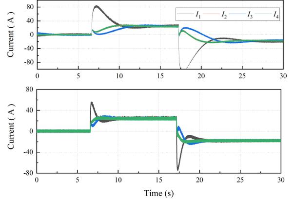
Fig. 11. Virtual state variables convergence speed tests when (a)  $a=10$  (b)  $a=100$
