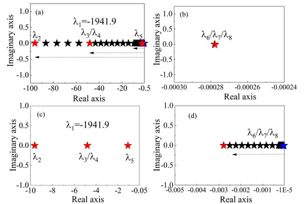
Fig. 6. Eigenvalue movement (a)  $\lambda_1$  to  $\lambda_5$  as  $a$  increases (b)  $\lambda_6$  to  $\lambda_8$  as  $a$  increases (c)  $\lambda_1$  to  $\lambda_5$  as  $k$  increases (d)  $\lambda_6$  to  $\lambda_8$  as  $k$  increases
