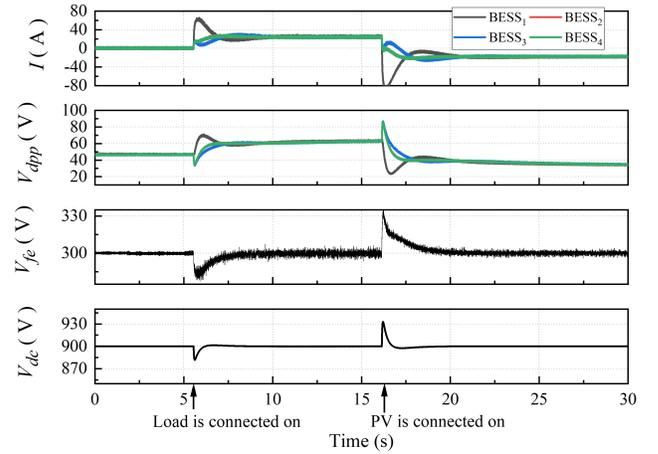
Fig. 8. Test results under load and PV disturbances
