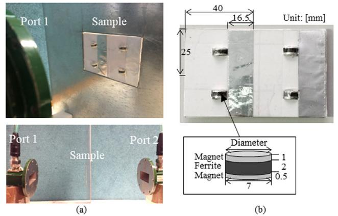
Fig. 2 Experimental setup (a) and 2×2 array sample (b)
