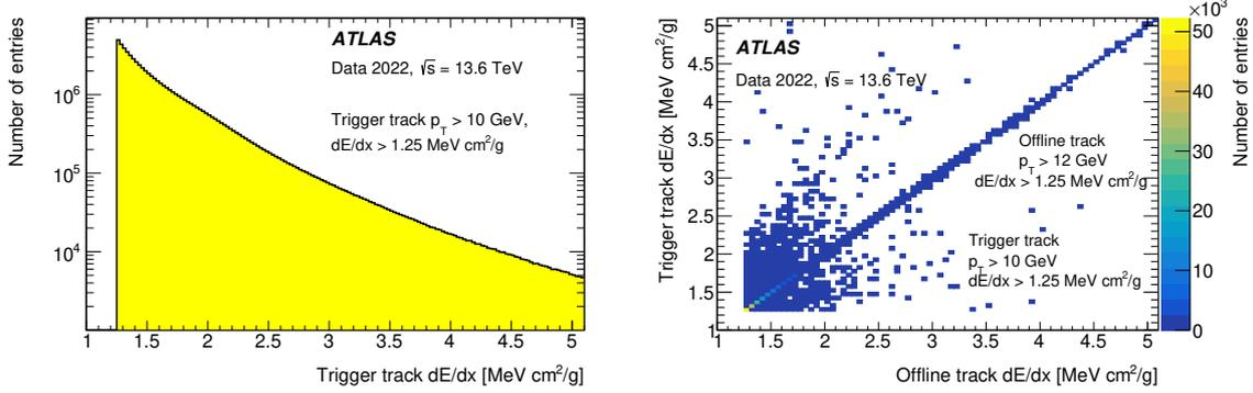
**Figure 55.** (Left) Distribution of  $dE/dx$  for tracks reconstructed in the trigger used for monitoring the  $dE/dx$ -based trigger. (Right) Correlation of online vs. offline  $dE/dx$  for offline tracks with  $p_T > 12$  GeV.
