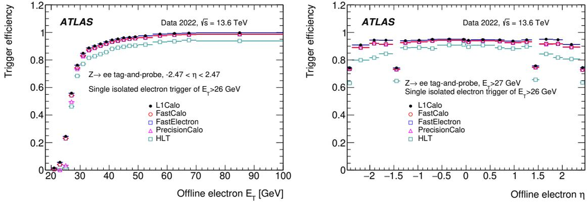
**Figure 33.** Efficiency of the primary isolated electron trigger with  $E_T > 26$  GeV for all steps of the HLT electron reconstruction as a function of the offline electron (left)  $E_T$  and (right)  $\eta$ . Efficiency is given with respect to the offline electrons which satisfy the tight identification and isolation criteria. Only statistical uncertainties are shown.
