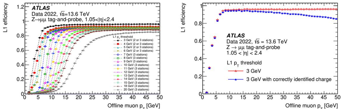
**Figure 4.** (Left) Efficiency of L1 muon triggers in the endcap region for various  $p_T$  thresholds. (Right) The efficiency of the charge identification for L1 muons with  $p_T > 3$  GeV. Only statistical uncertainties are shown.
