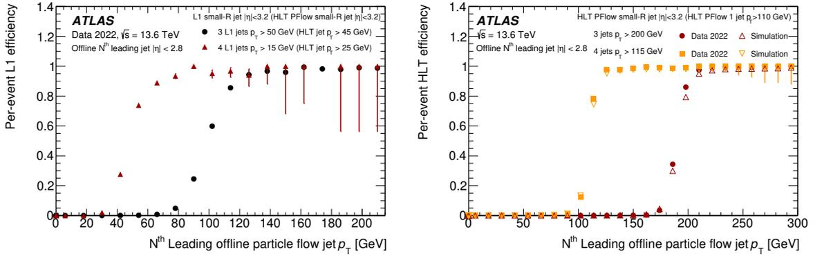
**Figure 43.** Multi-jet trigger efficiency as a function of the offline reconstructed  $N^{\text{th}}$  jet  $p_T$  (left) at L1 and (right) in the HLT. The efficiency is computed using the bootstrap method with respect to events taken by an independent single jet trigger, shown in brackets, that is 100% efficient in the relevant region. Only statistical uncertainties are shown.
