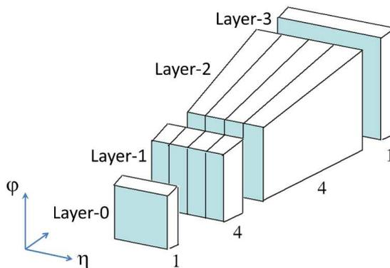
**Figure 2.** The trigger granularity from each  $0.1 \times 0.1$  trigger tower after the upgrade of the LAr Calorimeter electronics. Ten  $E_T$  values are provided from “1-4-4-1” longitudinal/transverse samples, each forming a SuperCell.
