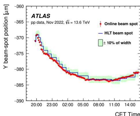
**Figure 63.** Time evolution of the vertical beam-spot position over the course of one LHC fill. The dots represent the monitored beam-spot position measured in luminosity blocks. The line represents the position currently used by the HLT algorithms which is measured as an average over a sliding window of a series of luminosity blocks. The band indicates a range corresponding to 10% of the vertical beam-spot width that was measured at the same time.
