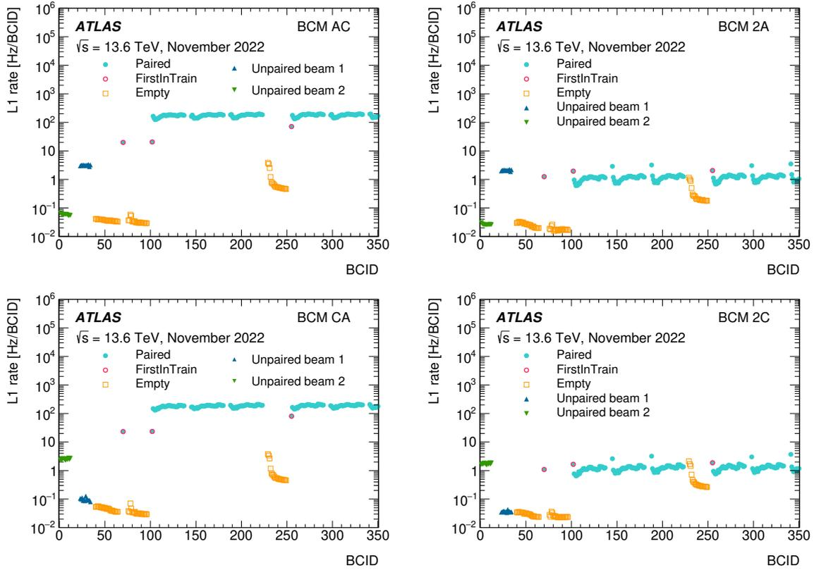
**Figure 62.** Per-BCID L1 rate of BCM hit-based triggers based on coincidence of (top left) AC and (top right) 2A, and (bottom left) CA and (bottom right) 2C. The per-BCID rates are shown for paired colliding bunches, the first colliding bunches in a train, empty bunch crossings (orange), unpaired bunch crossings with either beam 1 or beam 2 filled with a proton bunch. The BCID range shown is restricted to the first 350 BCIDs.
