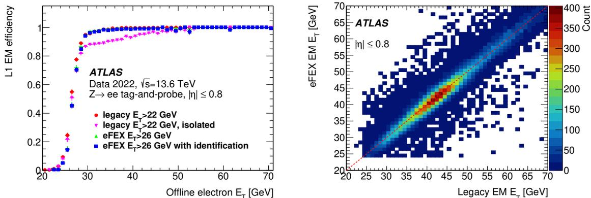
**Figure 3.** (Left) Efficiency of the L1 single-object electromagnetic (EM) trigger and (right) the correlation of the L1Calo transverse energies measured by the legacy Cluster Processor system and the Run-3 eFEX. Both measurements are done in the inner EM barrel within  $|\eta| < 0.8$ . Isolated legacy trigger [5] and eFEX trigger with identification [3] have the same rate. Only statistical uncertainties are shown.
