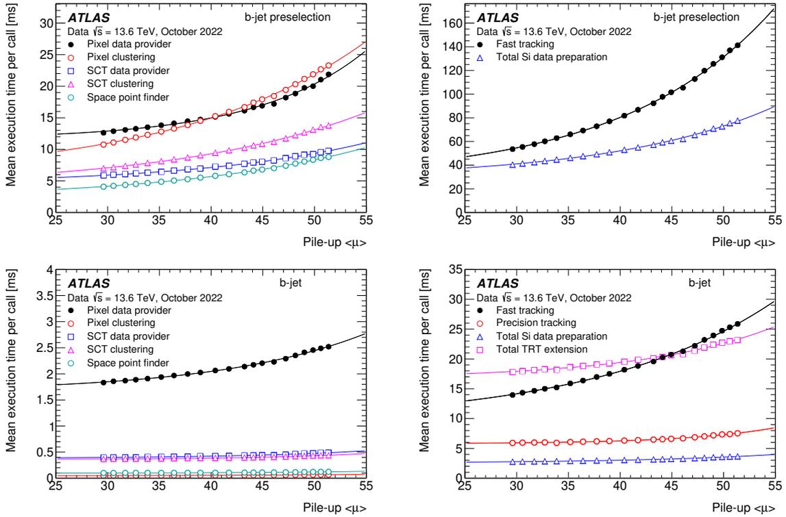
**Figure 25.** Execution times for data preparation, tracking, and TRT extension for (top) the  $b$ -jet preselection tracking and (bottom)  $b$ -jet RoI as a function of the average pile-up. The detailed breakdowns of the silicon data preparation components are shown on the left. Solid lines show ad hoc fits to data to guide the eye. Only statistical uncertainties are shown.
