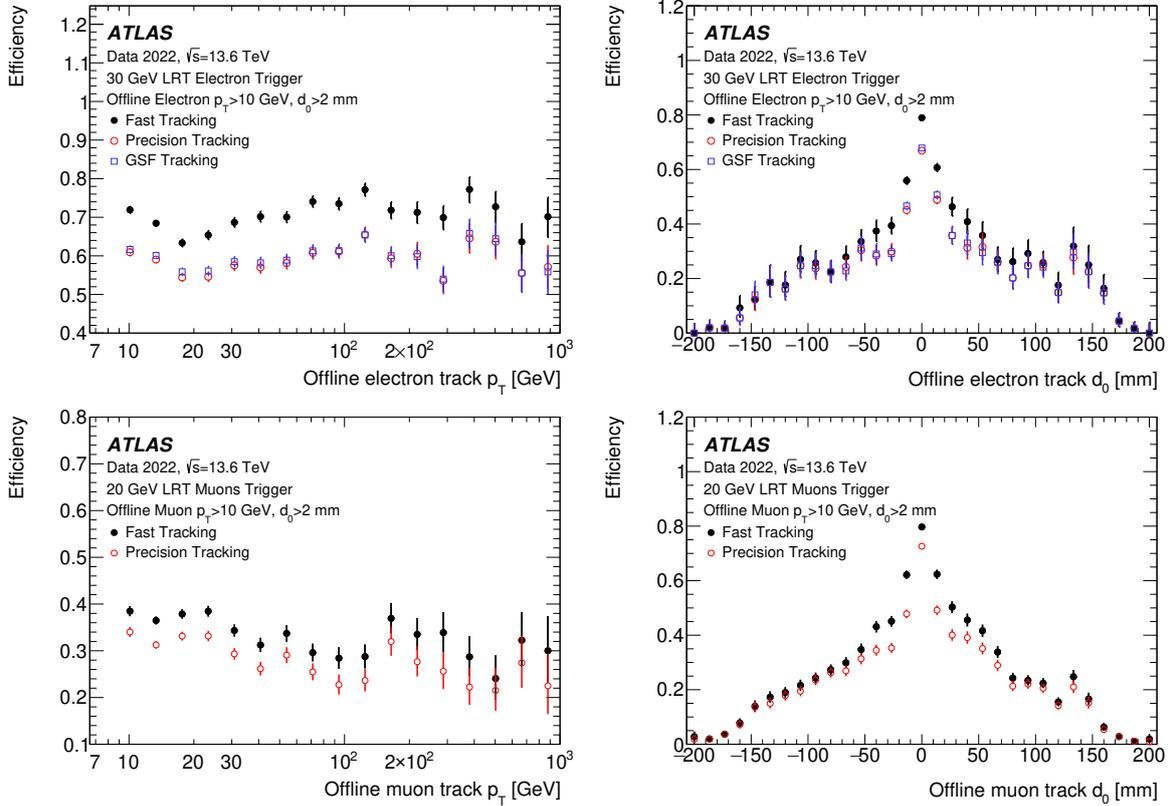
**Figure 17.** Fast and precision LRT efficiencies for (top) electron and (bottom) muon triggers as a function of offline electron and muon (left) track  $p_T$  and (right)  $d_0$ . The corresponding merged collections of standard and large radius offline electron and muon tracks are used. The efficiency for the additional GSF step for electrons is also included. Only statistical uncertainties are shown.
