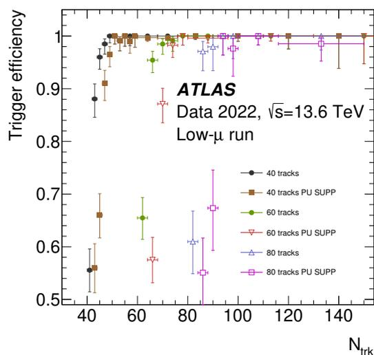
**Figure 53.** Efficiencies of high multiplicity triggers targeting selection of events with 40, 60, and 80 tracks as a function of number of tracks passing minimum-bias selection quality,  $N_{\text{trk}}$ . For each requirement the performance of the pile-up suppression (PU SUPP) variant of the trigger, designed to be robust in higher values of pile-up, is shown. Only statistical uncertainties are shown. These triggers were active during low pile-up runs in 2022.
