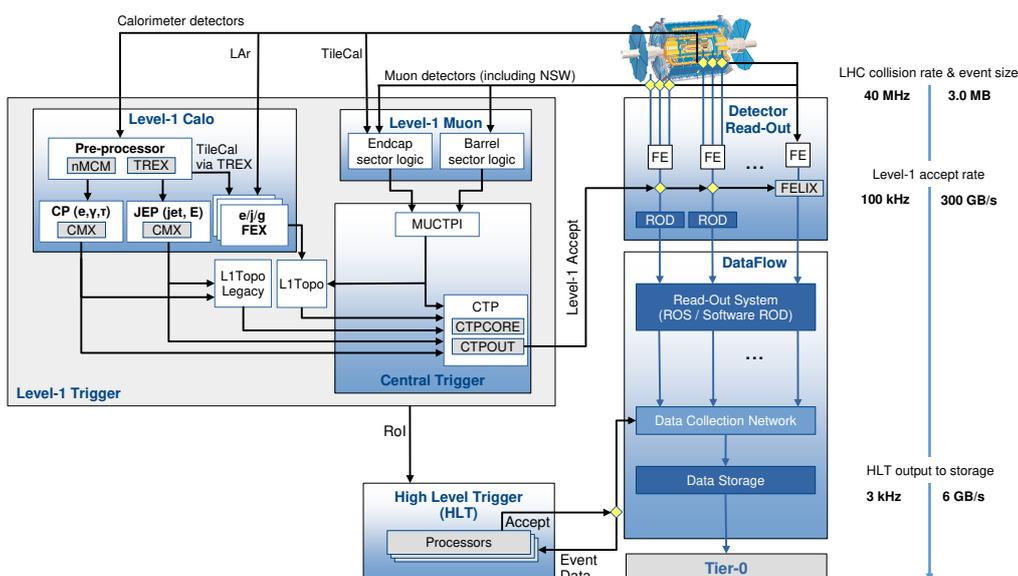
**Figure 1.** The ATLAS TDAQ system in Run 3 with emphasis on the components relevant for triggering as well as the detector read-out and data flow. Level-1 Calo, Level-1 Muon and the Central Trigger all send data to the Read-Out System (or FELIX/Software ROD), described in section 3.5, primarily for the purposes of offline validation and error checking. This is not shown in the diagram for simplicity. Abbreviations used are defined in sections 2.1 and 3.
