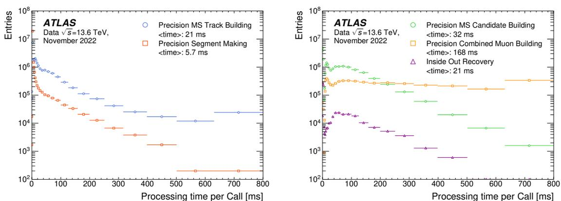
**Figure 32.** Processing times per ROI for the most CPU consuming precision steps: segment-finding and track-building algorithm (left), muon candidate building and inside-out recovery (right). The mean time of each algorithm is indicated in the legend. The last bin of the distributions includes the overflow events.
