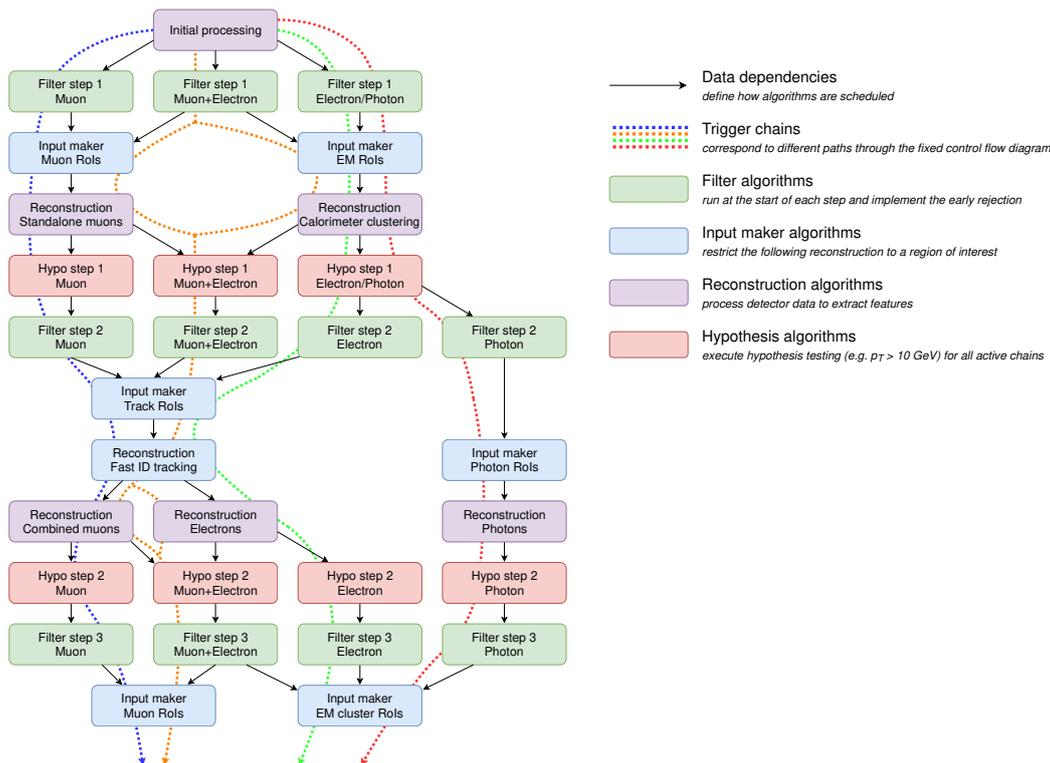
**Figure 7.** Example of control flow for menu processing. The control flow graph is created during initialisation and the steps are executed based on the available data. If a filter passes, processing continues through the next steps until all filters fail where the processing of the following steps is stopped. If the last step is reached with a chain passing all of its steps the event will be accepted.
