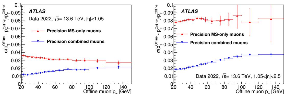
**Figure 30.** Width of the residuals for  $p_T$  as a function of the offline muon  $p_T$  for the precision MS-only and combined algorithms in (left) the barrel and (right) endcaps. Only statistical uncertainties are shown.
