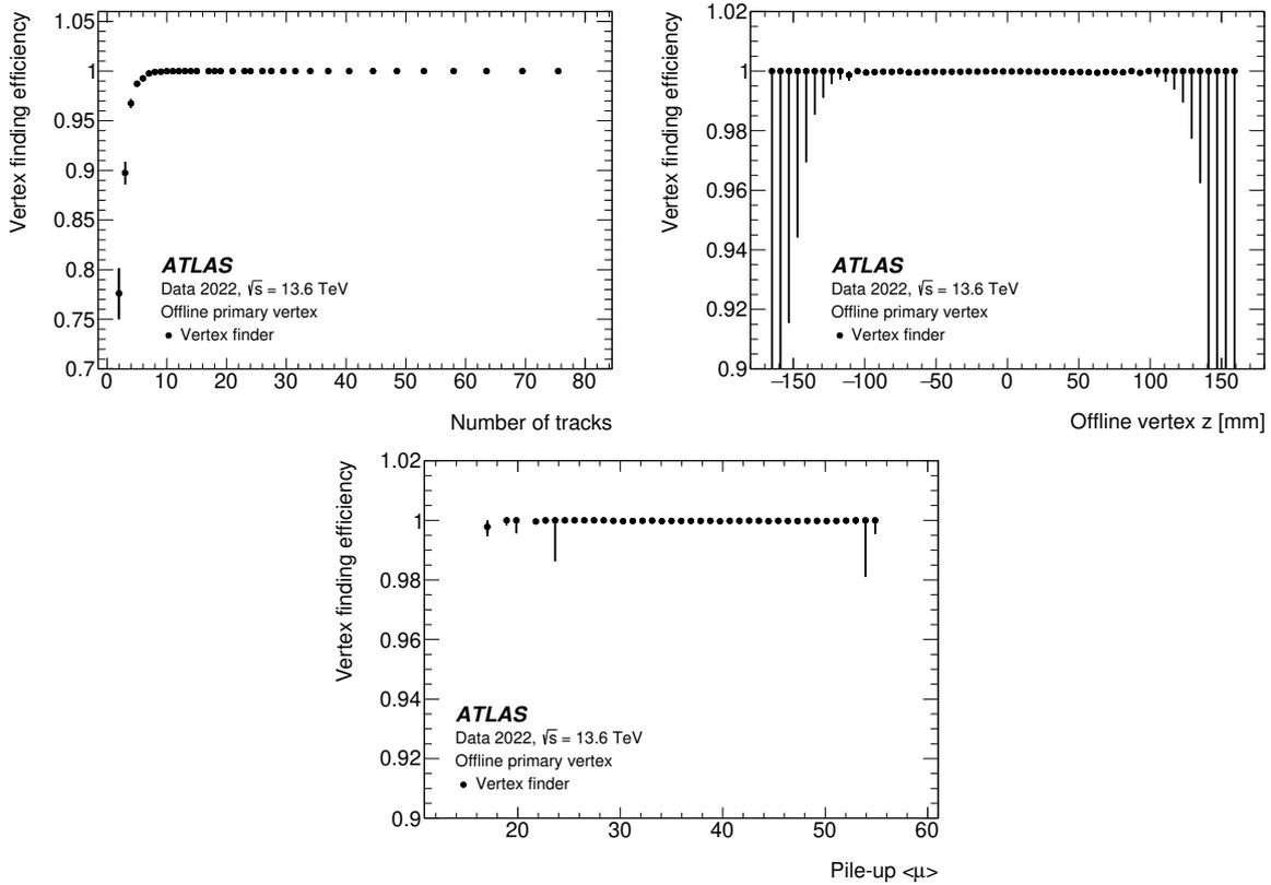
**Figure 14.** The trigger efficiency for finding the primary offline vertex, with respect to (top left) track multiplicity, (top right)  $z$  position, and (bottom) the average pile-up. The efficiency is evaluated for the 45 GeV jet trigger. Only statistical uncertainties are shown.
