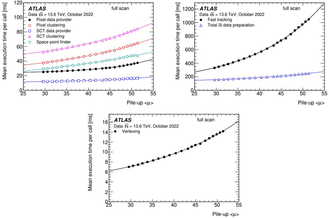
**Figure 24.** Execution times for (top left) the pixel and SCT data preparation, (top right) fast tracking and total silicon data preparation time for the full scan tracking in jet triggers, and (bottom) for the vertex finding with the full scan tracks, all shown as a function of the average pile-up. Solid lines show ad hoc fits to data to guide the eye. Only statistical uncertainties are shown.
