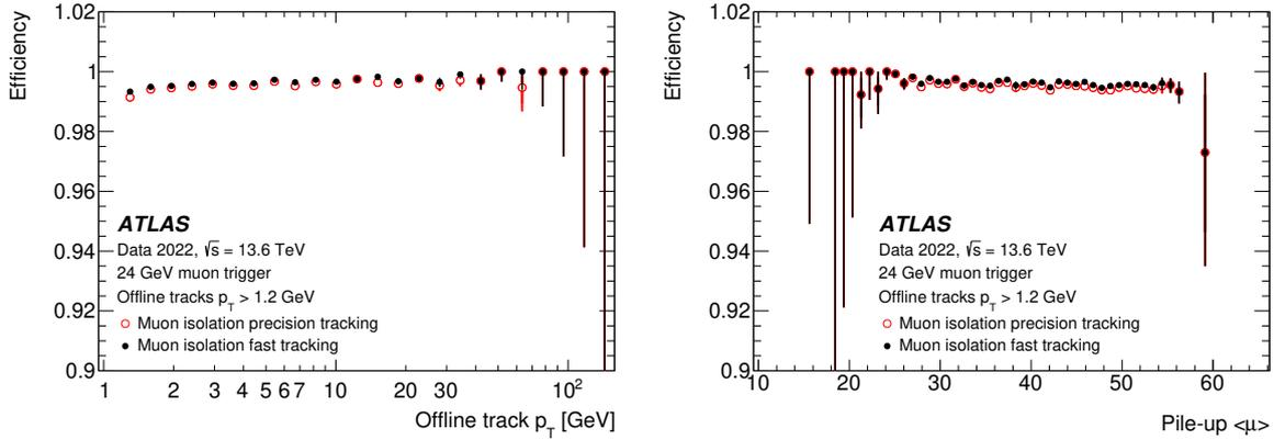
**Figure 10.** The tracking efficiency for non-muon tracks reconstructed in the *muonIso* RoI centred on the trigger muon selected by the 24 GeV muon performance trigger described in section 7.3, but without selection on the trigger tracks from the *muonIso* reconstruction. Efficiencies are shown for both the fast and precision tracking algorithms as a function of (left) the offline muon transverse momentum and (right) the average pile-up. Only statistical uncertainties are shown.
