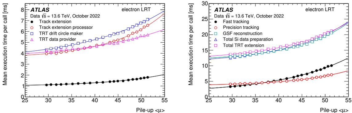
**Figure 27.** The TRT track extension, data preparation and tracking times for the electron large radius tracking algorithms as a function of the mean pile-up. The detailed breakdown of the TRT extension and data preparation stages are shown on the left, and the tracking times and combined silicon data preparation time and total TRT extension on the right. Solid lines show ad hoc fits to data to guide the eye. Only statistical uncertainties are shown.
