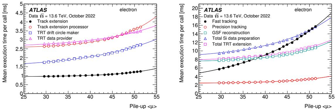
**Figure 23.** Execution times for the (left) TRT extension and (right) tracking and data preparation for the electron tracking, shown as a function of the average pile-up. Solid lines show ad hoc fits to data to guide the eye. Only statistical uncertainties are shown.
