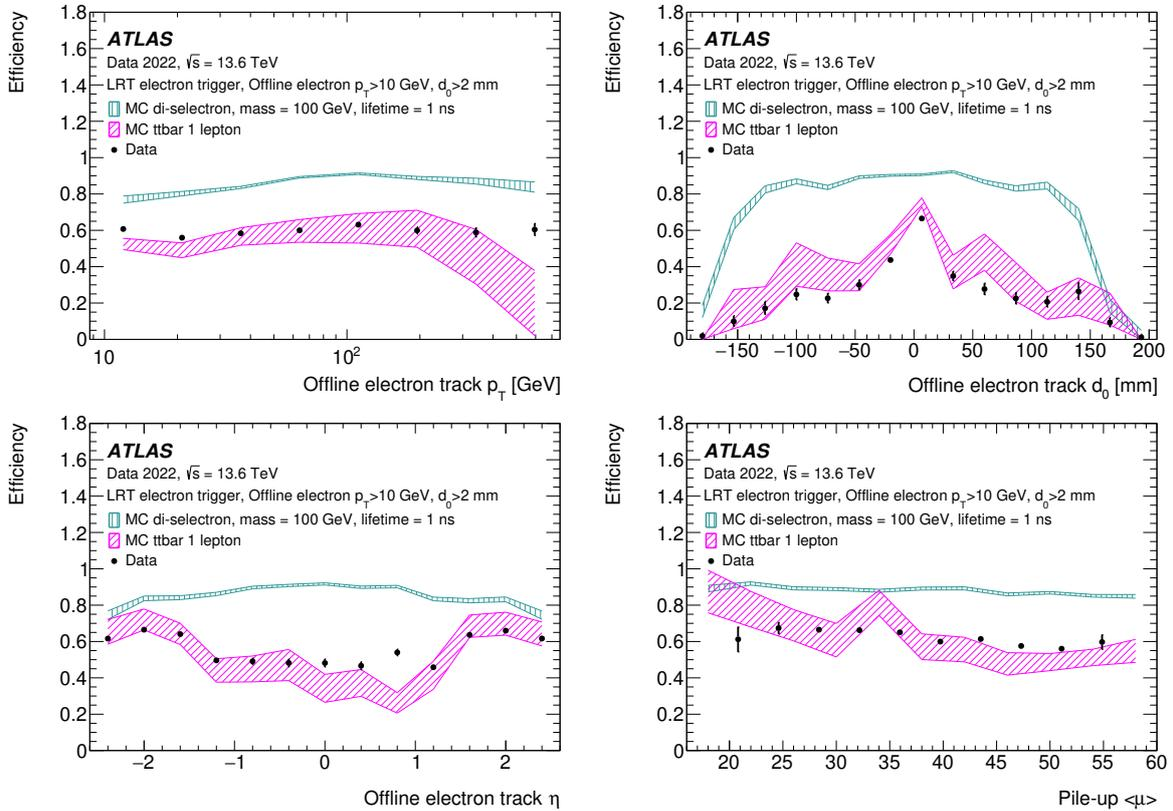
**Figure 18.** The GSF tracking efficiency for the LRT electron trigger with respect to the merged standard and large radius offline electron track collections versus (top left)  $p_T$ , (top right)  $d_0$ , (bottom left)  $\eta$ , and (bottom right) the average pile-up for data, semi-leptonic  $t\bar{t}$  MC events, and simulated pair production of selectrons with a 1 ns lifetime and a mass of 100 GeV. Only statistical uncertainties are shown.
