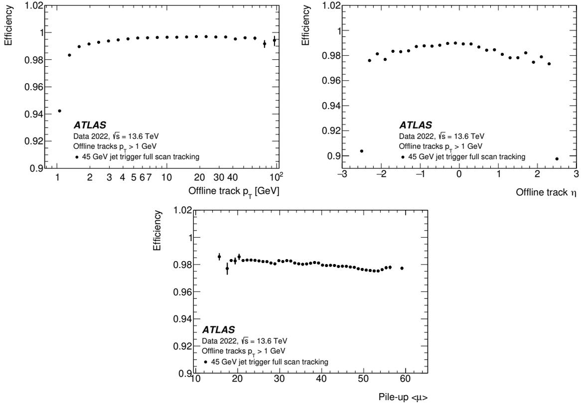
**Figure 13.** The full scan track finding efficiency with respect to offline tracks versus the offline track (top left)  $p_T$ , (top right)  $\eta$ , and (bottom) the average pile-up. The efficiency is evaluated for the 45 GeV jet trigger. Only statistical uncertainties are shown.
