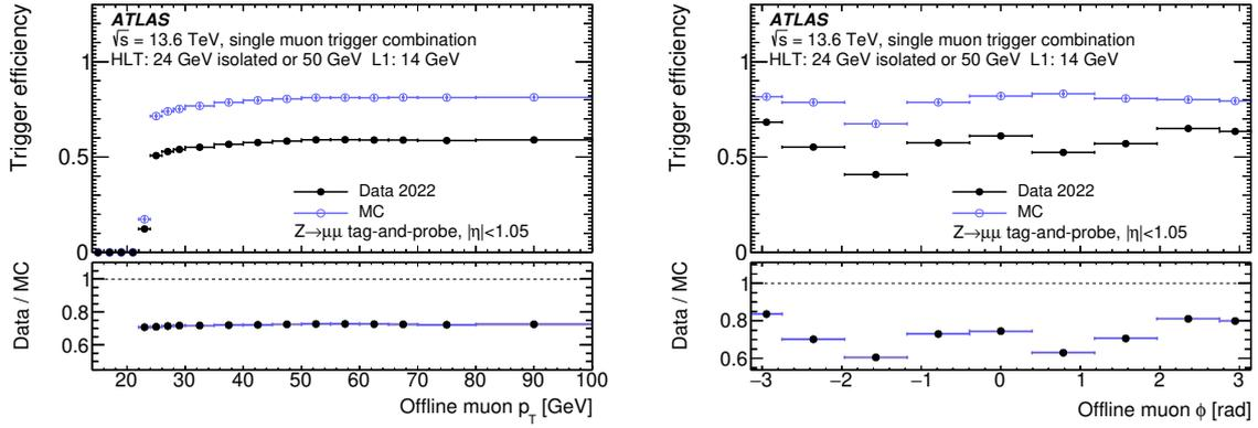
**Figure 37.** Muon trigger efficiencies as a function of (left)  $p_T$  and (right)  $\phi$  for  $p_T > 25$  GeV of the offline medium muon for the combination of two single-muon triggers in the barrel region. The ratios of data to MC simulation efficiencies are also shown. Only statistical uncertainties are shown.
