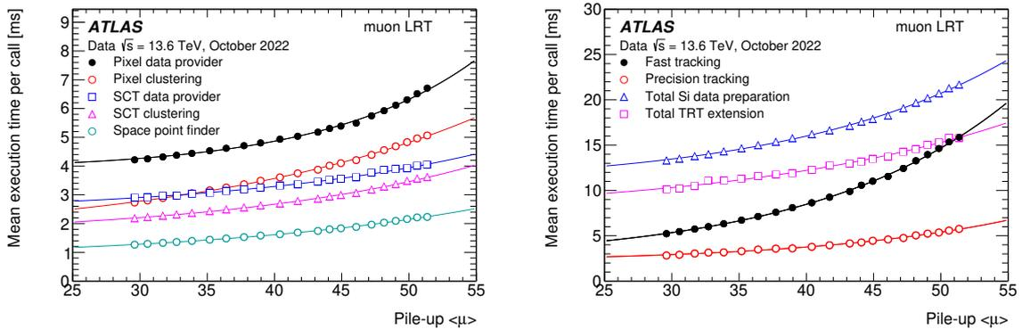
**Figure 26.** The data preparation, TRT track extension, and tracking times for the muon large radius tracking algorithms as a function of the mean pile-up. The detailed breakdown of the pixel and SCT data preparation stages are shown on the left, and the tracking times and combined silicon data preparation time and total TRT extension on the right. Solid lines show ad hoc fits to data to guide the eye. Only statistical uncertainties are shown.
