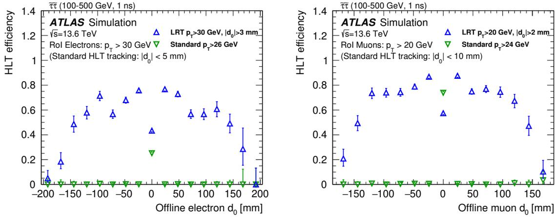
**Figure 59.** Displaced (left) electron and (right) muon trigger efficiencies with respect to their L1 seeds versus the offline lepton  $d_0$  (LRT, open triangles). The efficiencies for the isolated primary single electron and muon triggers (Standard), described in sections 6.1.2 and 6.2.1, are shown as inverted triangles. MC simulation samples with Run-3 conditions are used. Only statistical uncertainties are shown.
