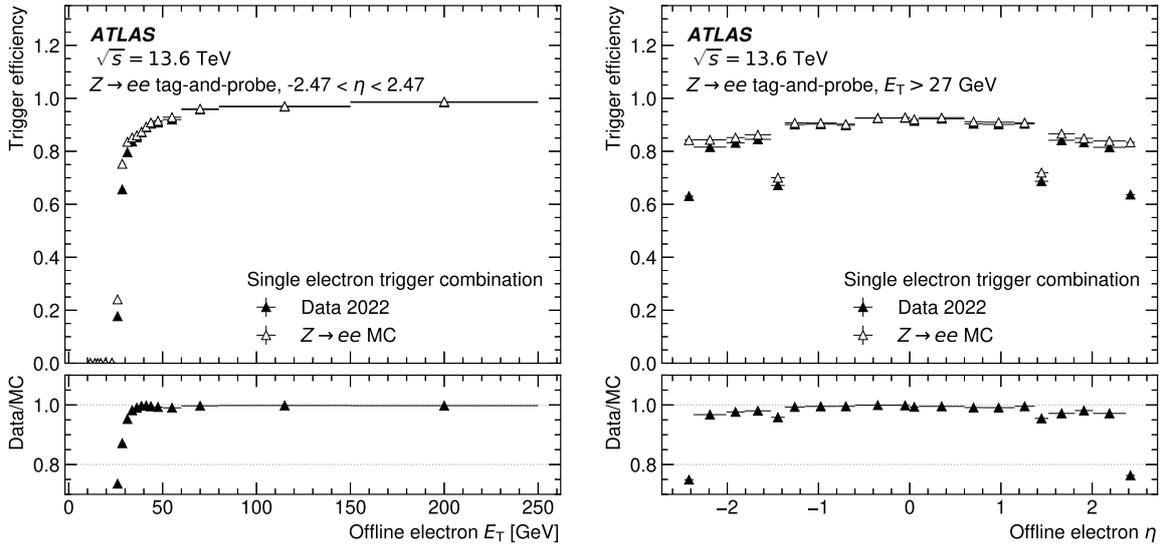
**Figure 34.** Combined efficiency of three primary single electron triggers as a function of the offline electron (left)  $E_T$  and (right)  $\eta$  for both MC simulation and 2022 data. Efficiency is given with respect to the offline electrons which satisfy the tight identification and isolation criteria. Only statistical uncertainties are shown.
