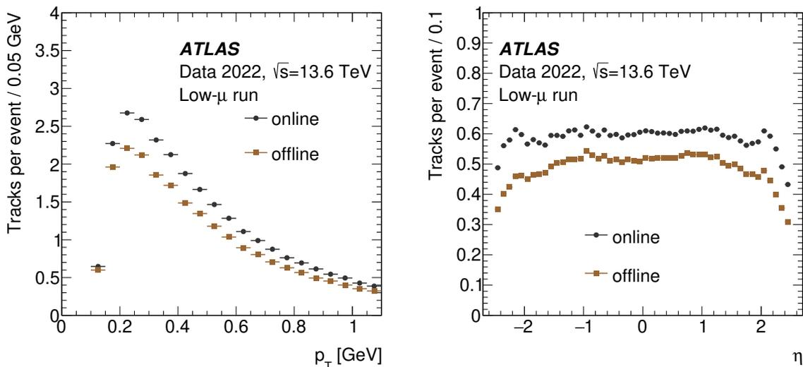
**Figure 51.** Comparison of (left)  $p_T$  spectra and (right)  $\eta$  of tracks reconstructed offline and passing minimum-bias quality selection and tracks reconstructed by the HLT online during low pile-up run in 2022.
