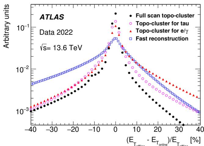
**Figure 28.** Transverse energy resolution in percent for HLTCalo clusters obtained with respect to calorimeter clusters reconstructed offline for 2022 data for the following algorithms: full scan topo-cluster for jets and  $E_T^{\text{miss}}$ , topo-cluster in RoI for taus, topo-cluster in RoIs for electrons (e) and photons ( $\gamma$ ), fast sliding-window reconstruction for  $e/\gamma$ .
