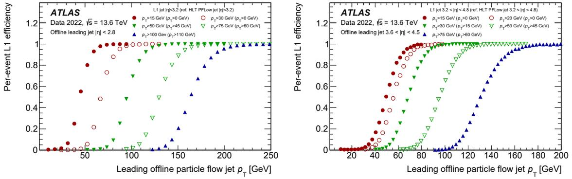
**Figure 41.** Efficiency of the legacy L1 single jet triggers in the (left) central and (right) forward regions. The efficiency is computed using the bootstrap method with respect to events taken by an independent trigger, shown in brackets, that is 100% efficient in the relevant region. Only statistical uncertainties are shown.
