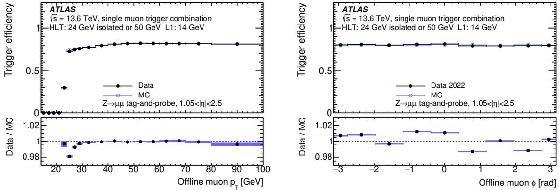
**Figure 38.** Muon trigger efficiencies as a function of (left)  $p_T$  and (right)  $\phi$  for  $p_T > 25$  GeV of the offline medium muon for the combination of two single-muon triggers in the endcap region. The ratios of data to MC simulation efficiencies are also shown. Only statistical uncertainties are shown.
