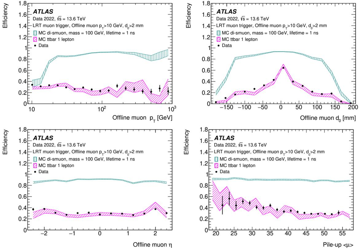
**Figure 19.** The precision tracking efficiency for the LRT muon trigger with respect to the merged standard and large radius offline muon track collections versus (top left)  $p_T$ , (top right)  $d_0$ , (bottom left)  $\eta$ , and (bottom right) the average pile-up for data, semi-leptonic  $t\bar{t}$  MC events, and simulated pair production of smuons with a 1 ns lifetime and a mass of 100 GeV. Only statistical uncertainties are shown.
