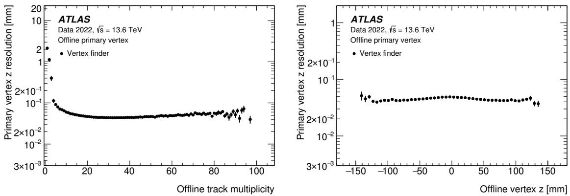
**Figure 15.** The resolution of the primary trigger vertex with respect to the primary offline vertex (left) track multiplicity and (right)  $z$  position. The efficiency is evaluated for the 45 GeV jet trigger. Only statistical uncertainties are shown.
