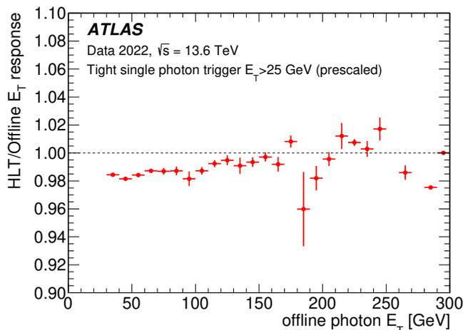
**Figure 36.** Energy response in TLA photons spatially matched to the leading offline photons. HLT-level photons are calibrated with the default sequence employed within the HLT reconstruction for the 2022 data taking, while reference offline photons are calibrated according to the Run-2 recommendations [44]. Events are required to satisfy a 25 GeV tight single-photon prescaled support trigger. Only statistical uncertainties are shown.
