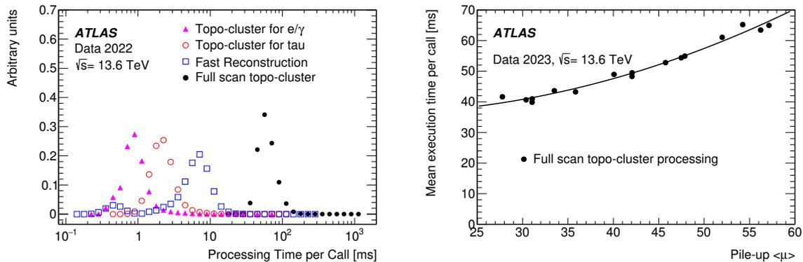
**Figure 29.** (Left) Processing time per call for the following algorithms: topo-cluster in RoIs for  $e/\gamma$ , topo-cluster in RoIs for taus, fast sliding-window reconstruction for  $e/\gamma$ , full scan topo-cluster for jets and  $E_T^{\text{miss}}$ . (Right) Processing time as a function of the average pile-up for the full scan topo-cluster algorithm. A solid line shows an ad hoc fit to data to guide the eye.
