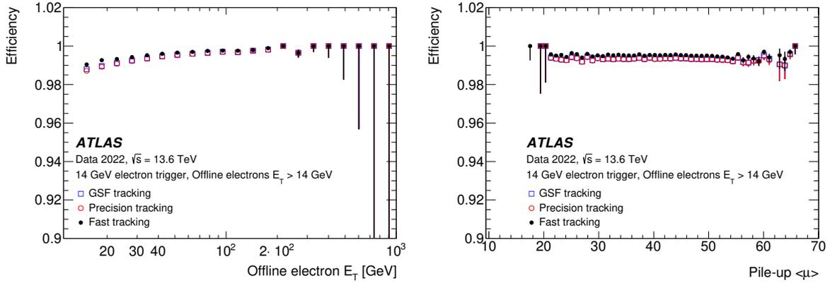
**Figure 11.** The ID tracking efficiency for electron candidates selected by the 14 GeV electron performance trigger described in section 7.3 which does not use ID tracking information. The efficiency with respect to offline electrons is shown as a function of (left) the offline electron transverse energy and (right) the average pile-up. Only statistical uncertainties are shown.
