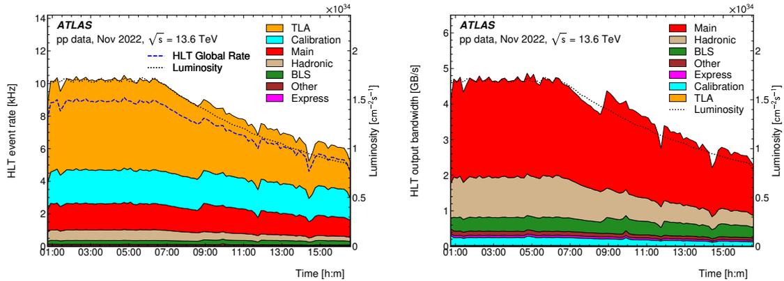
**Figure 8.** An example of (left) the rate and (right) bandwidth output by the HLT streams in a typical 2022  $pp$  run. The total HLT event rate is lower than the sum of the stream rates, because the same events may be written to multiple streams. The peak bandwidth of the TLA stream is approximately 25 MB/s, and consequently barely visible in the right hand figure. The event size per stream can vary up to a factor of 300.
