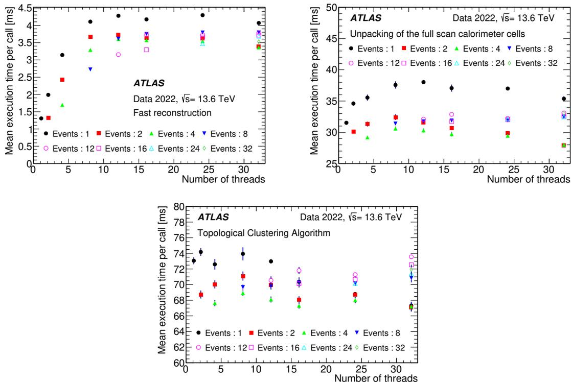
**Figure 65.** Mean execution time per call of (top left) the fast calorimeter reconstruction, (top right) the unpacking of the full scan calorimeter cells and (bottom) the full scan topo-clustering algorithm as a function of the number of threads for various numbers of concurrently processed events.
