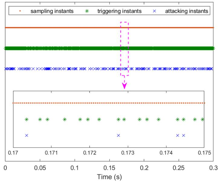
Figure 7: Triggering instants, attacking instants and sampling instants.
