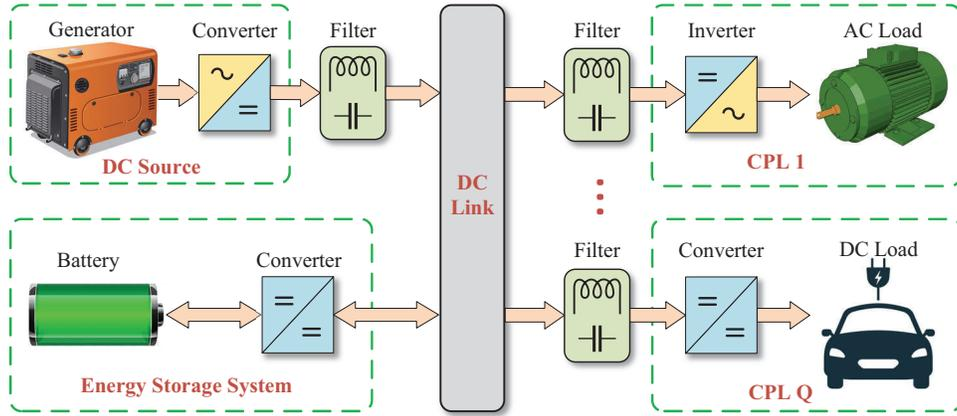
Figure 1: A DC microgrid with  $Q$  CPLs.
