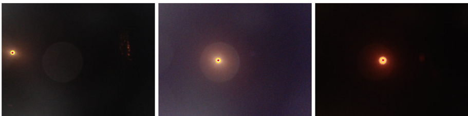
Fig. 6 Example images of the Sun SunbYte II. The red dot is the computation Sun centre for tracking. The yellow outer circle is the tracking of the Sun's edge
