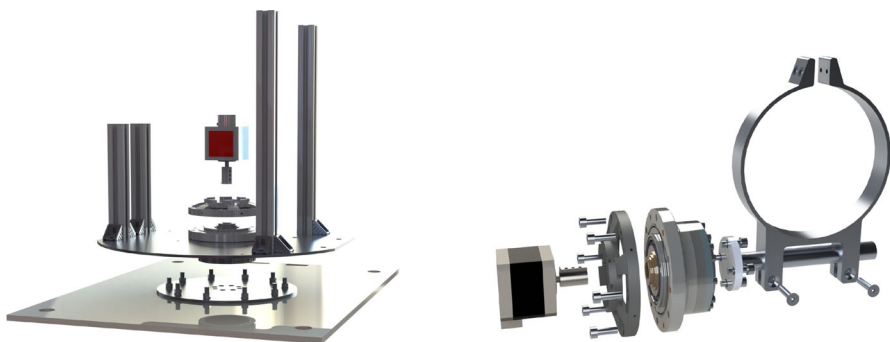
Fig. 4 Actuation line diagrams (right: Pitch, left: Yaw). The Yaw motor shaft is pointing downwards and rotates the base plate, this helps to reduce the total height of the system. The pitch motor is connected to the harmonic drive and the pitch clamp
