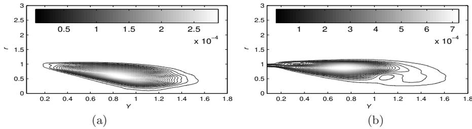
FIGURE 5. Contours of  $rI_{\omega}^{\text{LOW}}$  at  $St = 0.2$  and  $\theta = 30$  deg: (a) B118, (b) B122.
