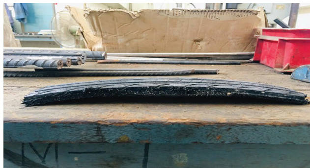
Figure 1: Tread sample for tensile strength test
