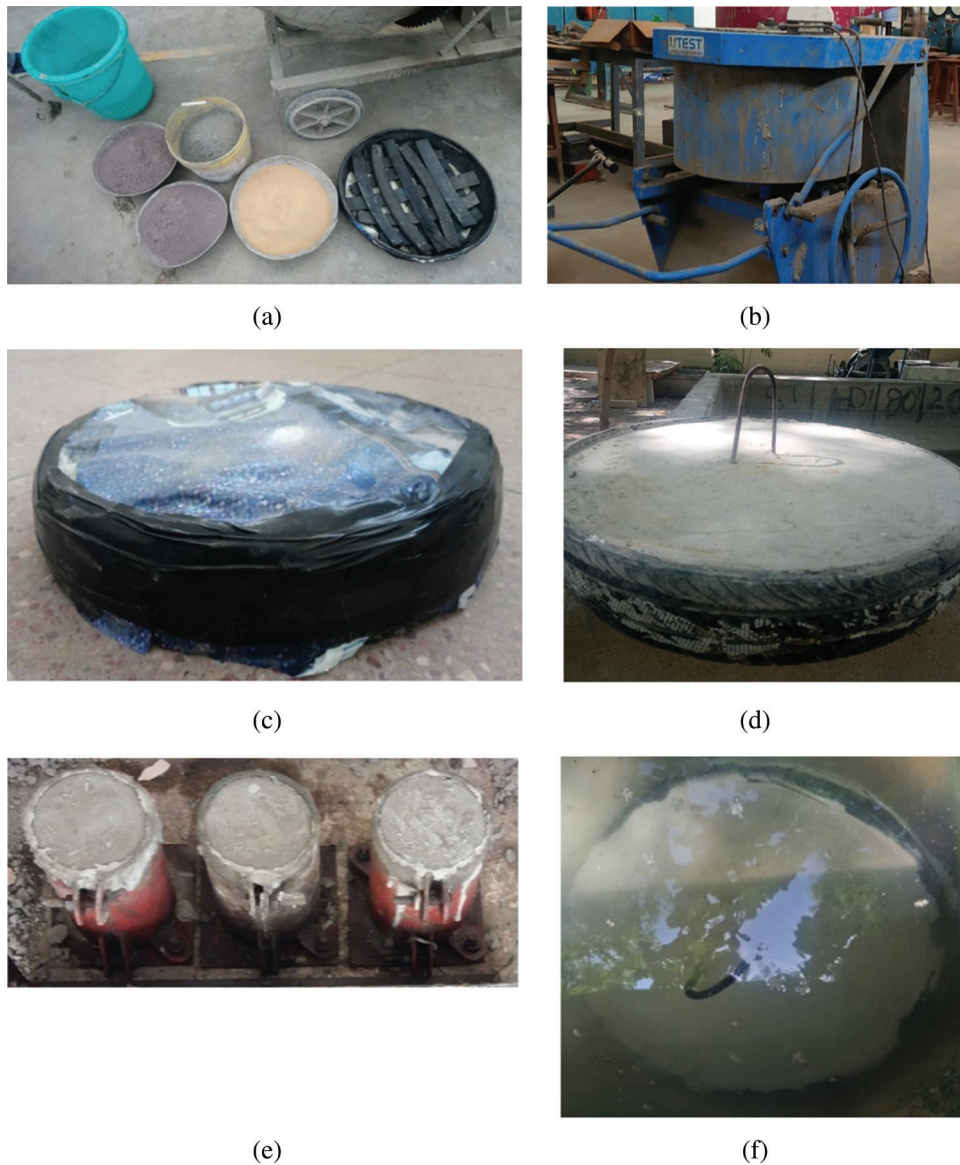
Figure 5: Mixing, casting and curing of specimens (a) All ingredients and mold for manhole cover (b) Pan mixer used (c) Inverted mold showing plastic for casting (d) Manhole cover sample after casting (e) Cylinder specimens (f) Curing of specimen
