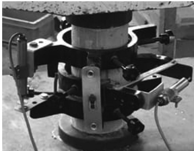
Figure 6: Cylinders tested under compression
