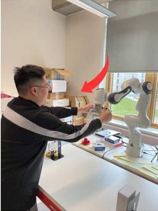
Fig. 5: An operator manually guiding the end effector of a Franka robot arm, indicated by the red arrow, to demonstrate the desired motion. This is essential for collecting human demonstrations for robotic training.
