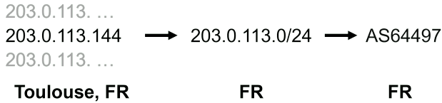
Figure 2: Inferring the location of an AS by propagating geolocation data. We propagate the location of IP addresses within the advertised prefixes of an AS to infer the physical location(s) of that AS. We do this both for the observed peer_ip in the global routing table, as well as separately for its advertised prefix ranges.
