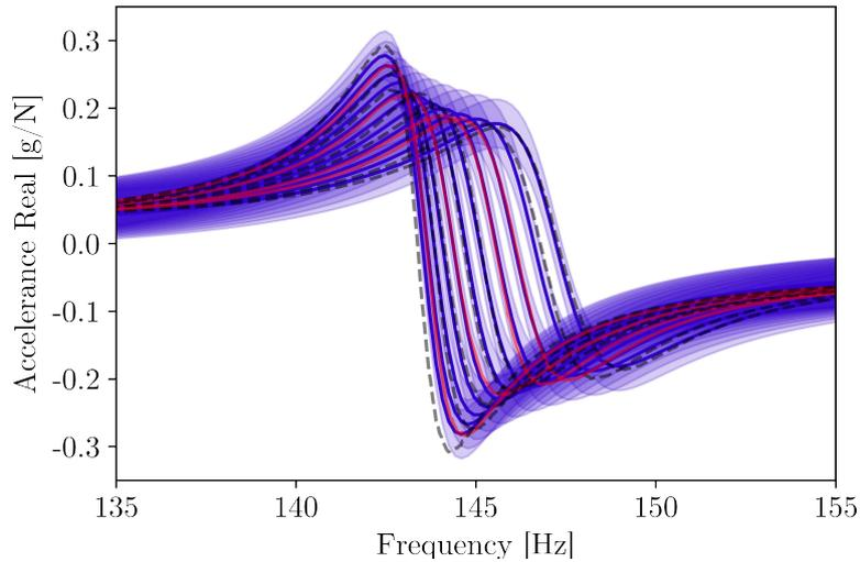
Figure 4. Extrapolated FRFs using population-level variables. The extrapolated means are shown as solid blue lines, with shaded blue regions indicating variance bounds (3-sigma deviation). Solid red lines are the FRFs used for training the model, while dashed black lines are the measured FRFs at ‘unseen’ temperatures.
