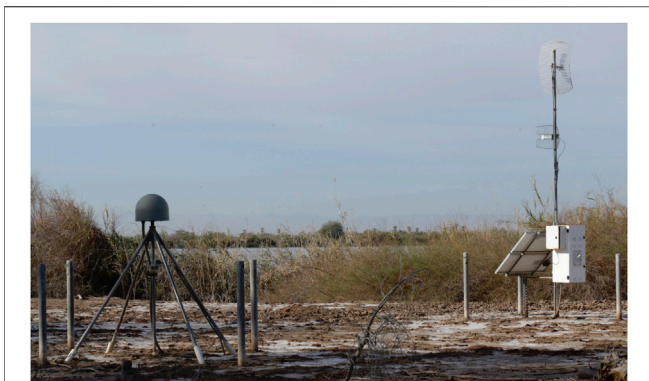
FIGURE 2 | Earthscope Consortium Plate Boundary Observatory (PBO) GPS (GNSS) network station at Ramer Lake, near Calipatria, CA [33.0814, -115.5102]. The view direction is towards a true bearing of 205°. This is a Geodetic Facility for the Advancement of Geoscience (GAGE) with additional data at: https://www.unavco.org/data/doi/10.7283/T59P2ZKG . Image © W Brian Whalley CC BY-NC-ND 4.0.
