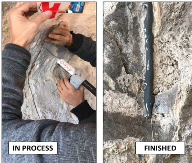
Fig. 7 The distributed fiber before and after gluing
