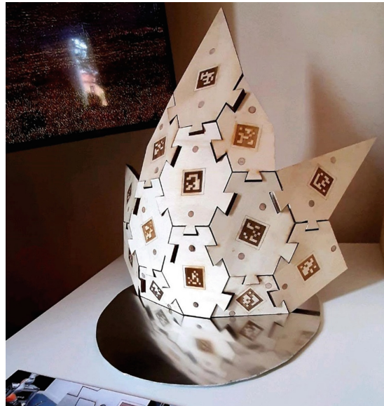
Fig. 5. The “Set in Transition” interlocking leaf structure. Each panel element is inserted along the vector perpendicular to its own plane.
