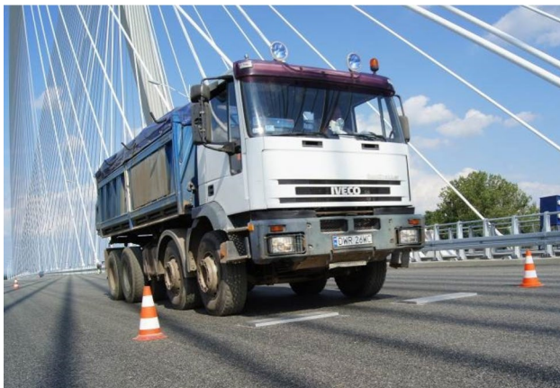
Fig. 2 A lorry driven over a bump during a proof loading test on the Rędziński Bridge in August 2011, after [29]
