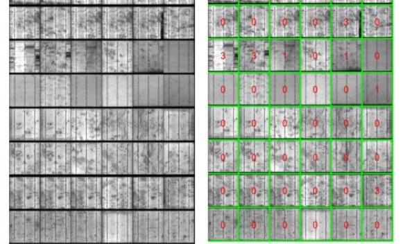
Figure 3. EL image before and after automated crack processing, with 0 indicating a healthy cell and 1-5 representing specific crack types (line cracks, soldering anomalies, complex cracks, Edge ribbon cracks, and PID).
