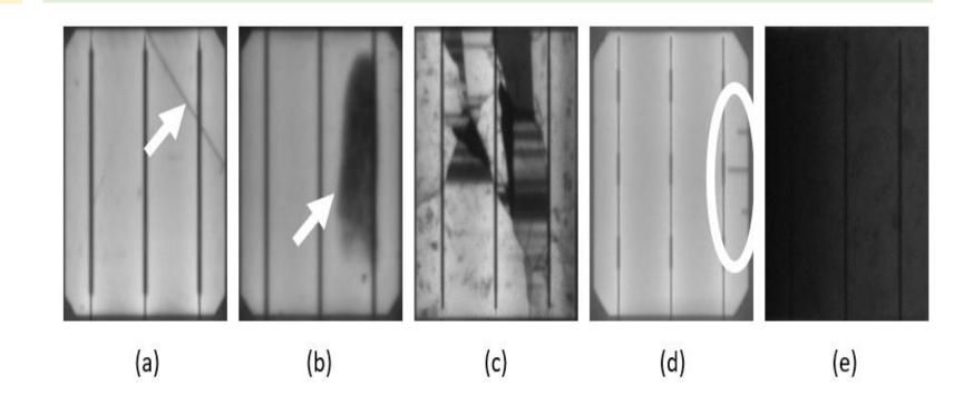
Figure 2. PV defect types investigated in this work: (a) Line cracks; (b) Soldering anomalies; (c) Complex cracks; (d) Edge ribbon cracks; (e) PID [2].
