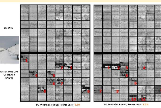
*Figure 7.* Impact of heavy snow on PV efficiency and cracks propagation.
