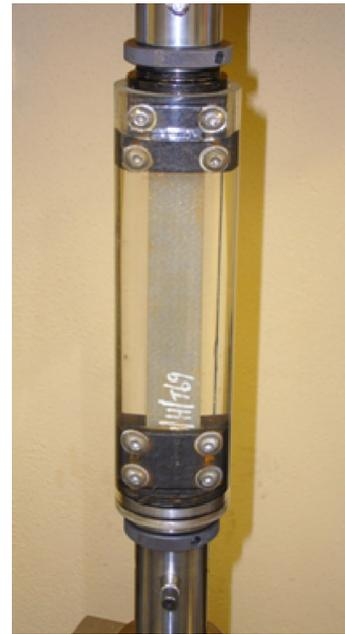
**Fig. 4** Immersed fatigue test setup, acrylic tube with O-ring seal
