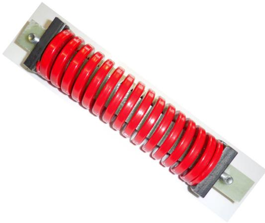
**Fig. 3** Stressing mechanism for stress ageing of GFRP coupon
