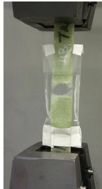
**Fig. 5** Immersed fatigue test setup, polyethylene pouch with waterproof tape
