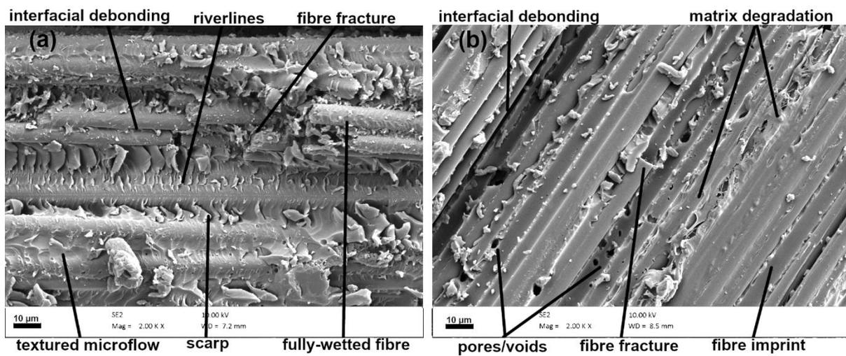
**Fig. 4.** High magnification (x2000) SEM micrographs of both the (a) dry and (b) wet UD 50C composites. The scale bar represents 10  $\mu\text{m}$ .
