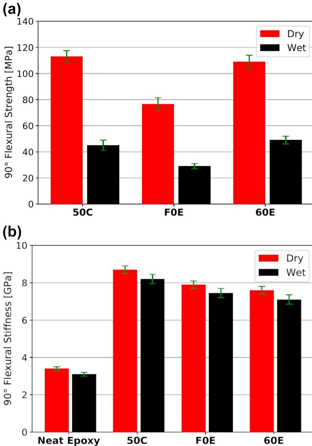
**Fig. 3.** Transverse flexural (a) strength and (b) stiffness results i.e., dry and conditioned cases, for the T700S family composites as well as for the neat (powder) epoxy blocks. The (90°) flexural values are averages from ~6 tests for each examined case. The obtained results were normalised at ~59% FVF for means of comparison.
