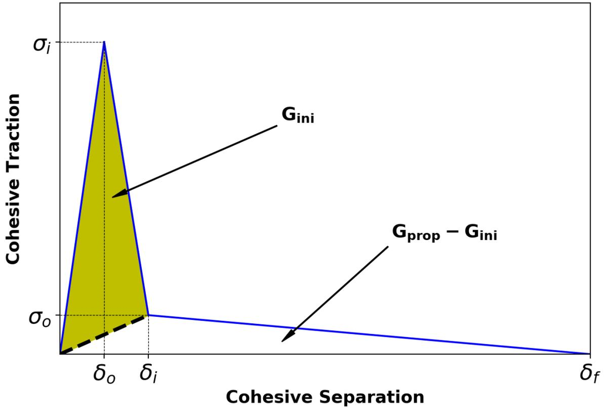
Fig. 10. Cohesive trilinear traction separation law, reproduced from [67].
