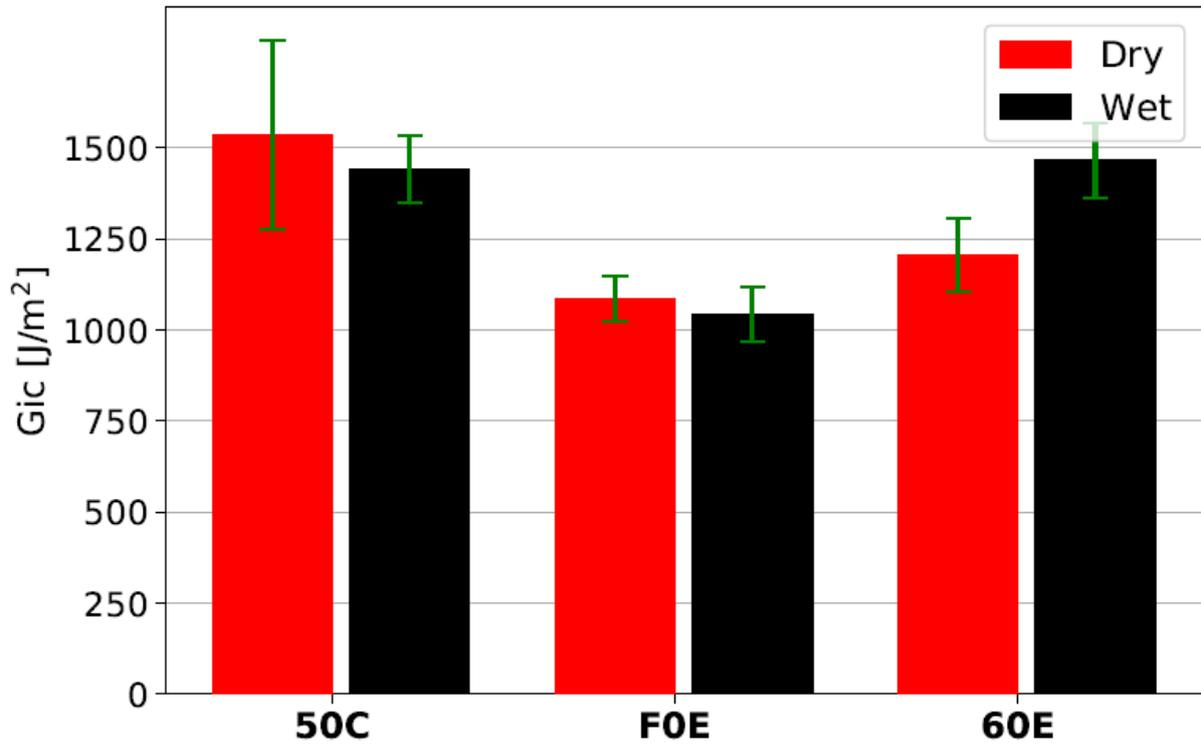
**Fig. 6.** Propagation  $G_{IC}$  for the Mode I DCB tests for all the composites cases. The values are calculated according to ASTM D5528 (MBT) and represent the average R-Curve values from the 5% compliance point until the end of the test.
