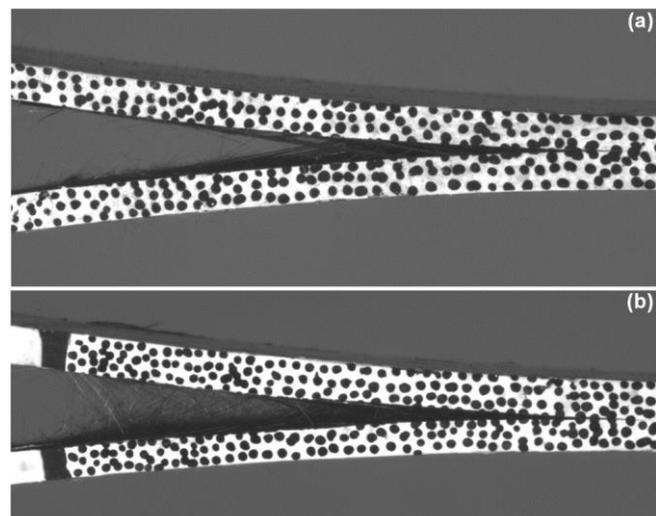
**Fig. 7.** High speed images of the crack tip zone in detail of 50C (a) dry composite and (b) immersed/wet case. Note that extensive fibre bridging can be observed for the wet CFRP case compared to dry sample.
