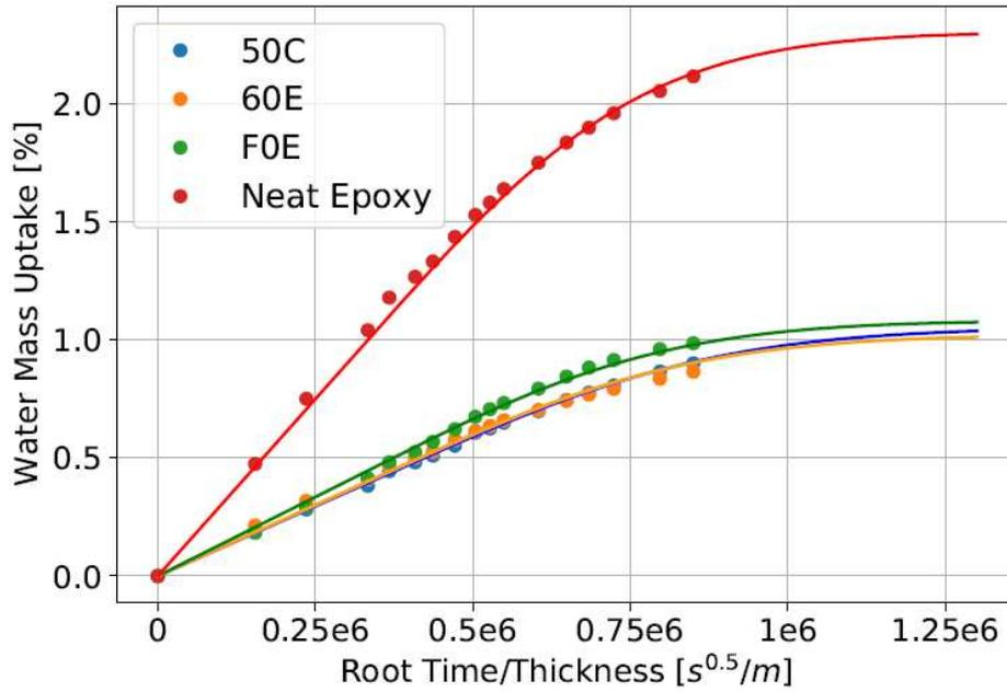
**Fig. 1.** Experimental moisture mass uptake of the three composite cases i.e., 50C, F0E and 60E, and the pure powder epoxy plate immersed in the seawater and plotted against the theoretical Fickian Diffusion Curves.
