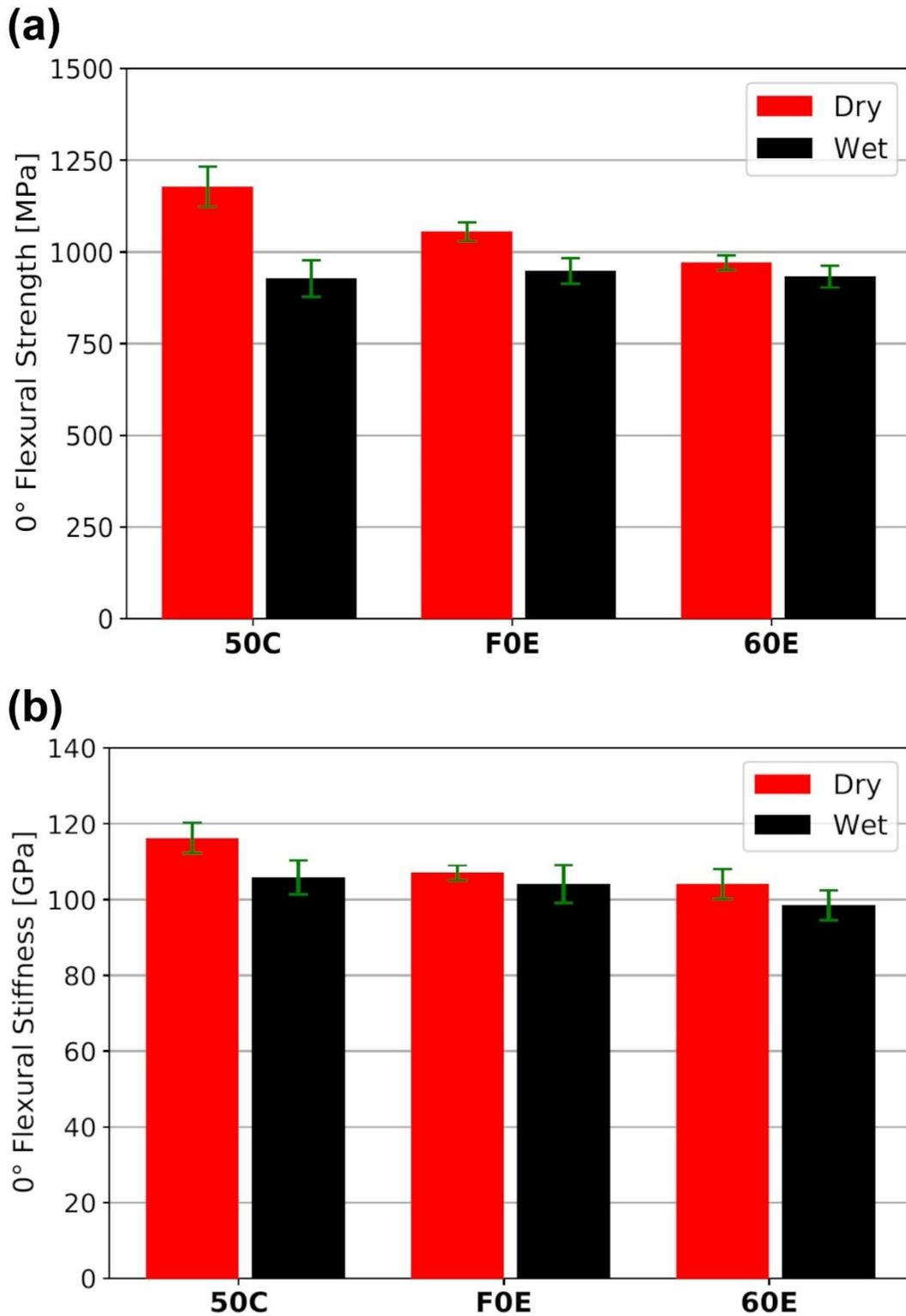
**Fig. 2.** Overall flexural results (a) strength and (b) modulus of the T700S composite family for the dry and immersed/wet cases. The longitudinal flexural results are average values from ~6 tests for each case i.e., dry and wet. The obtained results were normalised at ~59% FVF for means of comparison.
