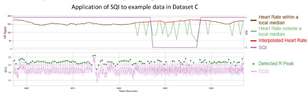
561 562 Figure 13. A demonstration of SQI on dataset C. Top: The derived HR signal. Brown and green 563 lines represent the raw HR. Brown HR is HR that falls within a local median, while green HR falls 564 outside the local median. The red HR line represents the HR following local linear interpolation to 565 remove outlier HR points. The purple line represents the SQI vector indicating whether a time 566 point has good (=1) or poor (=0) signal quality. This vector indicates a noisy period when the HR 567 data can be considered unreliable and thus excluded from further analyses. Bottom: The 568 corresponding ECG signal (light purple), with the detected R-peaks shown as green dots. 569 Individual missing peaks can be approximated by interpolation, but a noisier period (SQI=0) 570 becomes harder to recover and so is considered unreliable.
