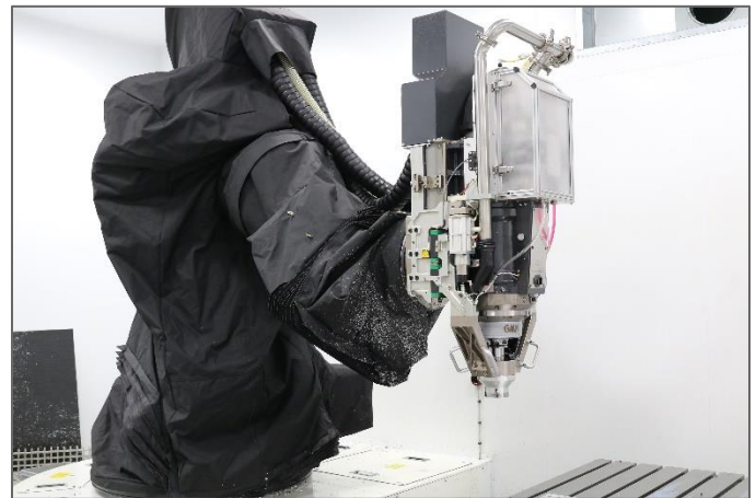
Figure 1. Accurate Robotic Milling System (ARMS).
