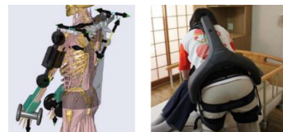
Fig 3.10 Medical worker exoskeleton optimised through musculoskeletal simulation.
