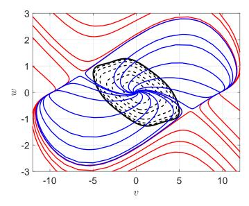
Figure 3. Estimate of the region of attraction  $(\mathcal{E}(V,\rho))$  (black solid) of the vehicle model of numerical example 4 obtained using the polynomial Lyapunov function of Proposition 1. Also shown are sublevel sets of the Lyapunov function (black dashed), stable trajectories of the system (blue) and unstable trajectories (red).
